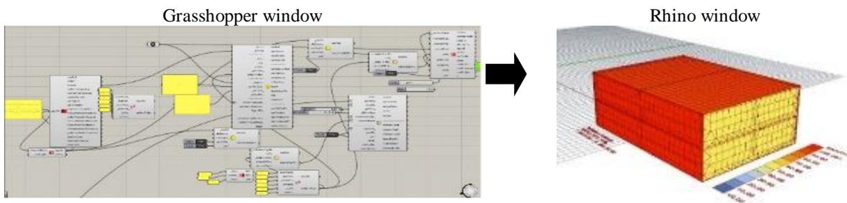
**Figure 2:** Shows work procedures in Grasshopper tool using Ladybug to build analysis network on the building casing, and results are presented on the Rhino window (by researchers)
