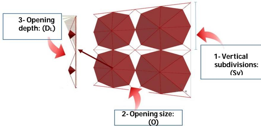
**Figure 6:** shows design parameters used to form the typical unit
