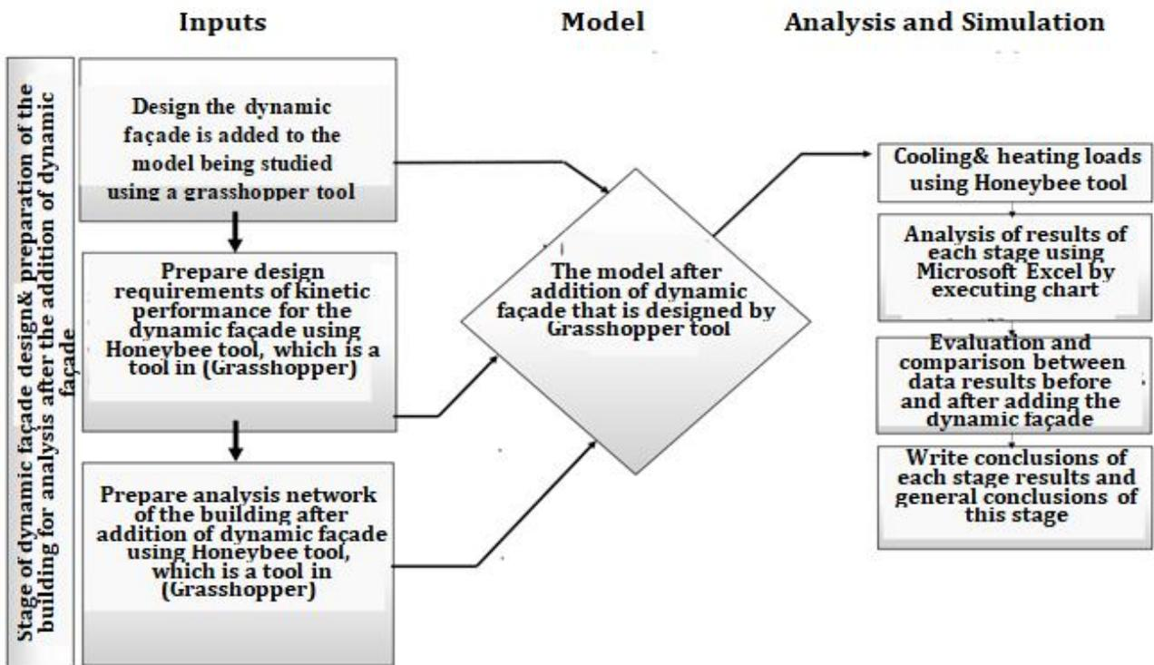
Figure 4: Shows a dynamic façade design methodology and evaluation using simulation programs. (by researchers)
