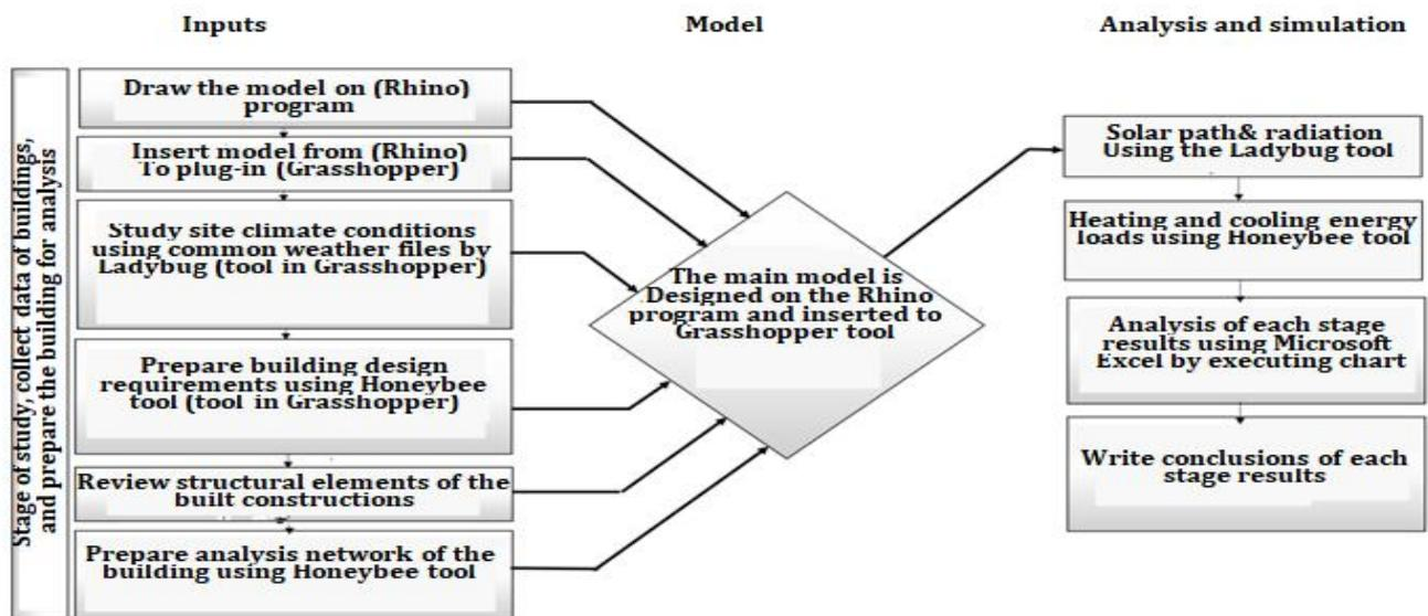
**Figure 1:** shows building design methodology and evaluation using simulation programs. (by researchers)
