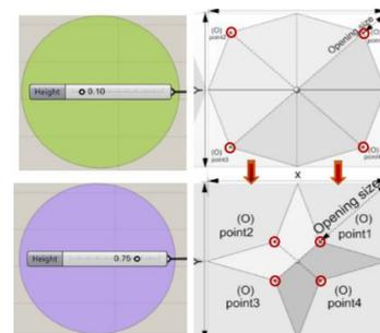
**Figure 8:** Points controlling the second parameter (opening ratio), (by researchers) .
