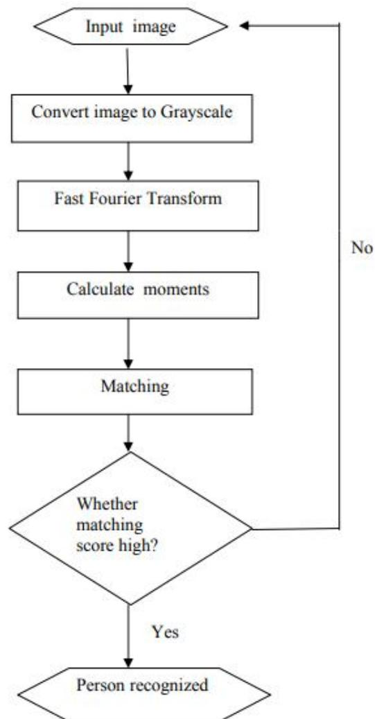
**Figure 4** Algorithmic steps for Iris Recognition System
