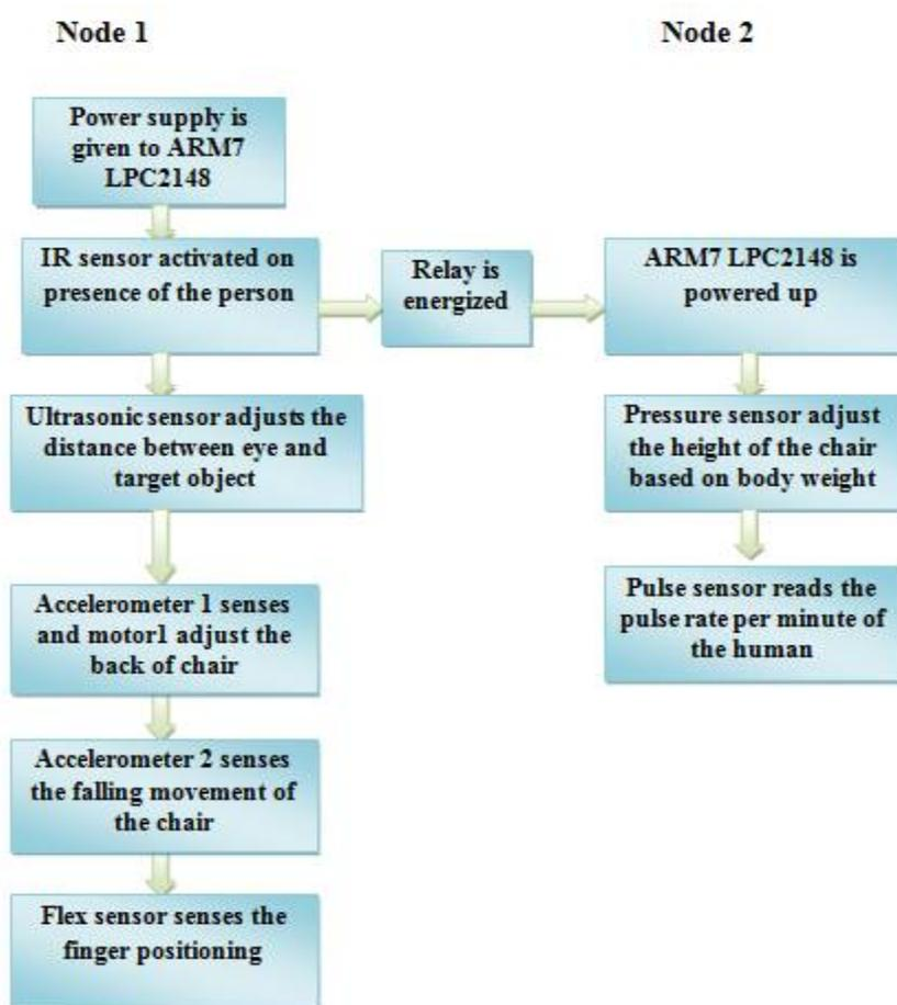
**Figure 3:** Graphical representation of functioning of smart chair.
