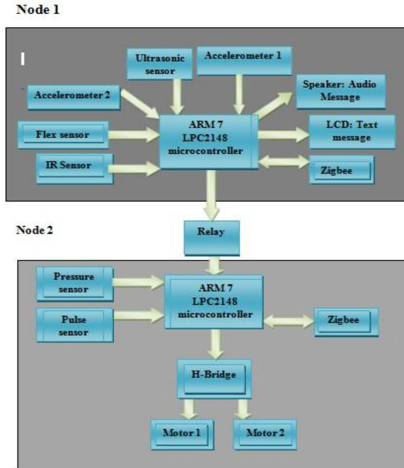
**Figure 1:** Block diagram of smart chair.
