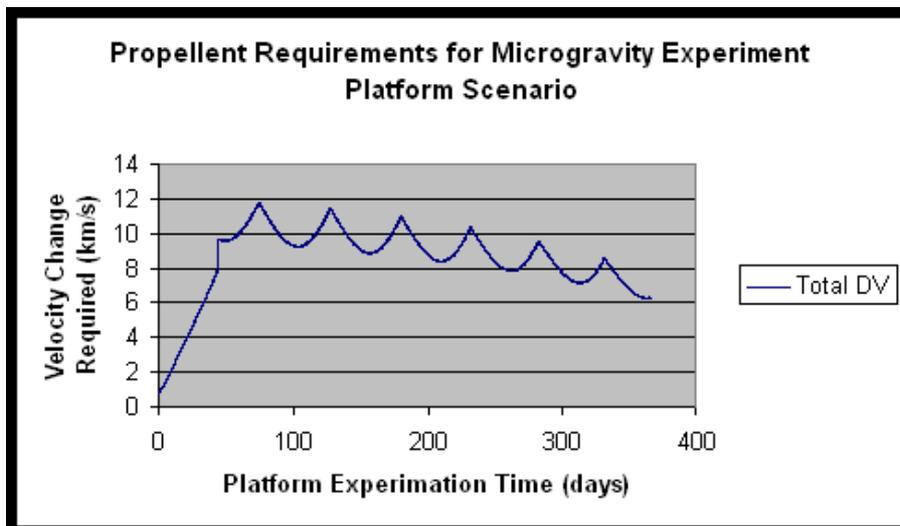
**Figure 3** SFU  $\Delta V$  required to complete scenarios up to a year away from station
