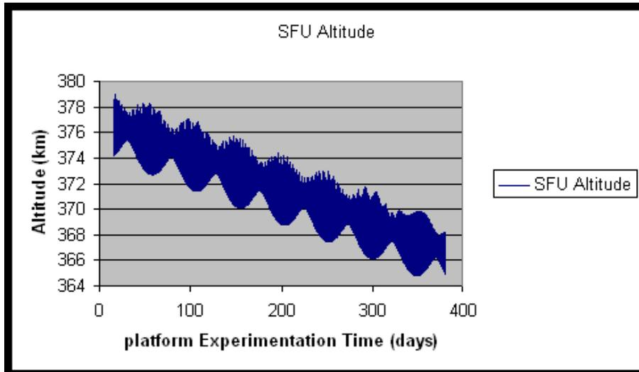
**Figure 2** SFU altitude for one-year simulation
