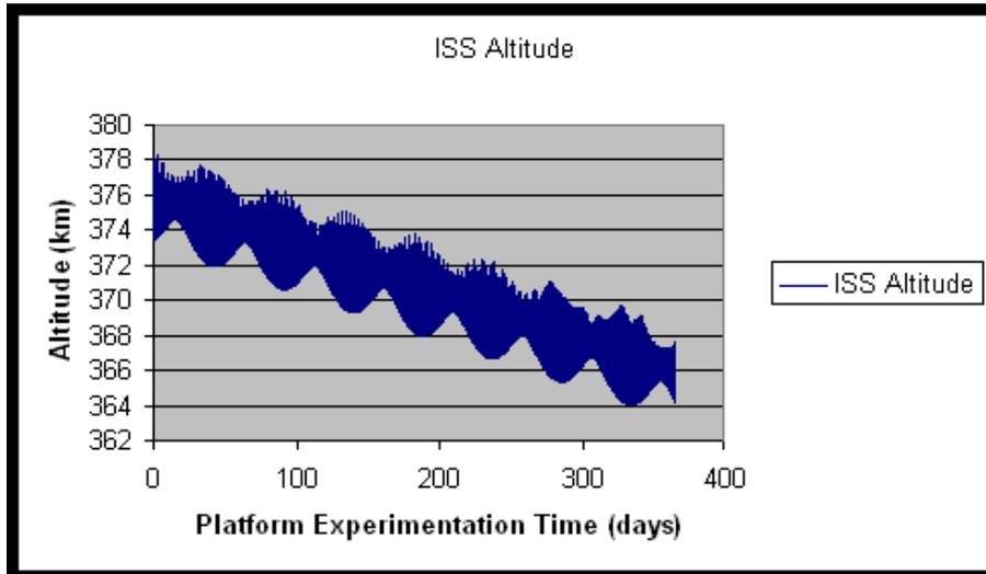
**Figure 1** ISS altitude for one-year simulation
