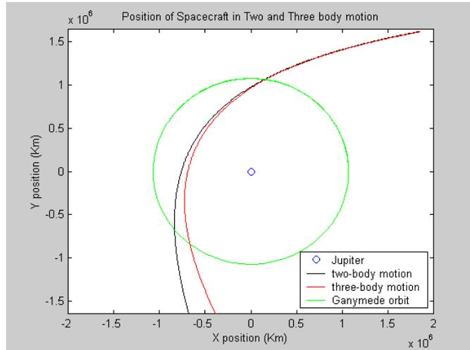
Figure 7 Europa Orbiter position in two and three body position
