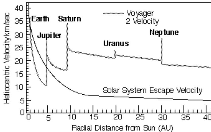
**Figure 1** Voyager 2 Gravity Assist Velocity Changes
