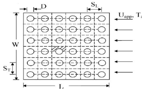
Fig 4.1: Schematic of in-line pin-fin heat sinks
