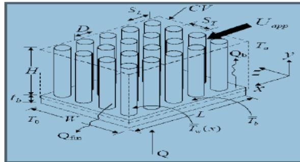
Fig 4.2. Geometry of in-line pin-fin heat sink
