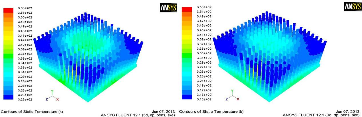
Fig 4.8: Temperature contours of splayed copper pin fin heat sink with 3 m/s velocity.
