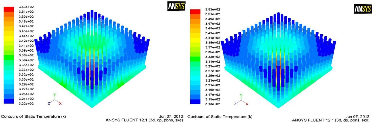
Fig 4.4 & Fig 4.5 Temperature contours of std aluminum pin fin and std. copper pin fin heat sink with 3 m/s velocity.
