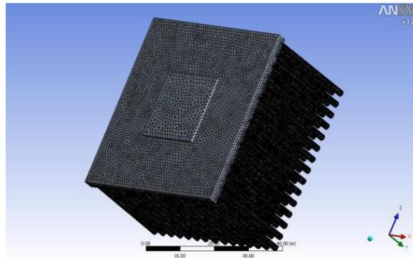
Fig 4.3. Meshing of In-Line Pin-Fin Heat Sink
