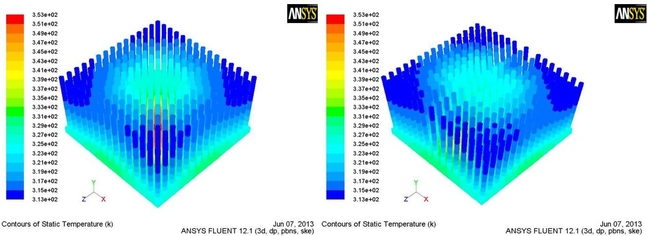
Fig 4.6: Temperature contours of standard hybrid pin fin heat sink (copper base plate with al heat sink) with 3 m/s velocity. And Fig 4.7: Temperature contours of splayed al pin fin heat sink with 3 m/s velocity
