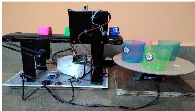
**Fig.14**The proposed automated colourbased customized product collation system
