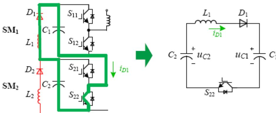
Fig. 7: Simplified circuit of SM1 and SM2
