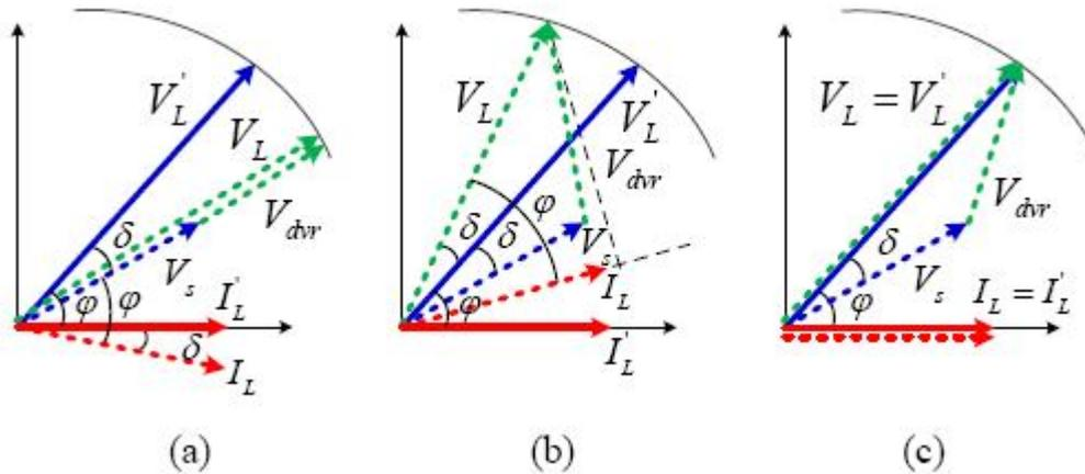
**Fig. 8: Phasor representations of the three basic strategies: (a) in-phase; (b) energy-optimized; (c) pre-sag.**
