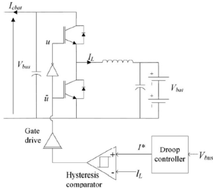
**Fig 3: Battery DC –DC converter**
