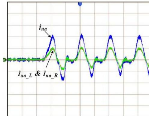
**Fig. 13: Experimental waveforms of the currents flowing through the left- and right-side cluster, and the whole arm.**
