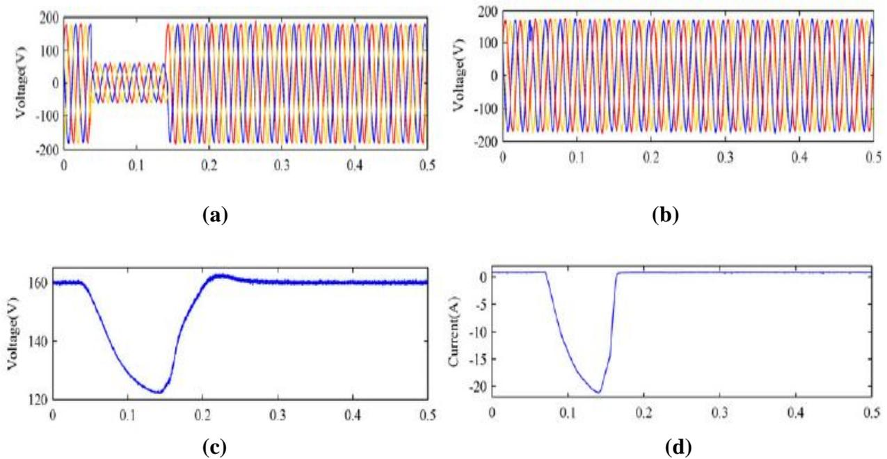
**Fig. 11. Battery System Experimental results: 0.1s Three phase sag to 35% of nominal voltage.**
