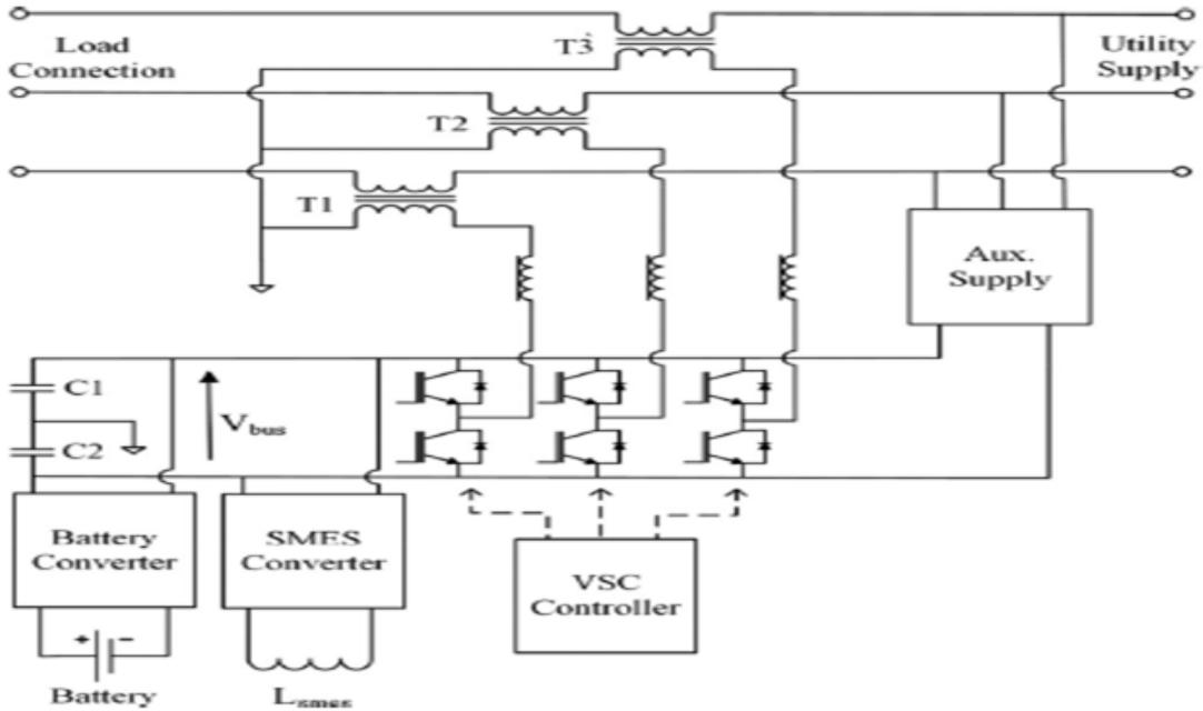
**Fig.1: Hybrid Energy DVR system configuration**
