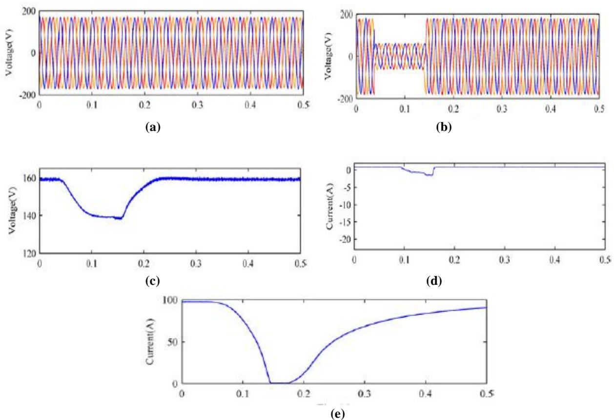
**Fig. 10: Hybrid System Experimental results: 0.1s Three phase sag to 35% of nominal voltage. (a) Supply voltages. (b) Load voltages (c) DC Link Voltage Battery Current (d) SMES-inductor current.**
