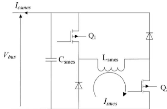
**Fig 2: SMES DC/DC converter**
