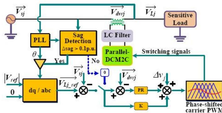
**Fig. 9: Control block of the proposed DVR system.**
