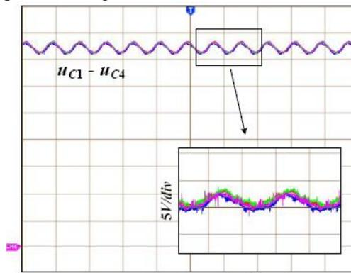
**Fig. 12: Experimental waveforms of the capacitor voltages in upper arm of the parallel-DCM2C.**
