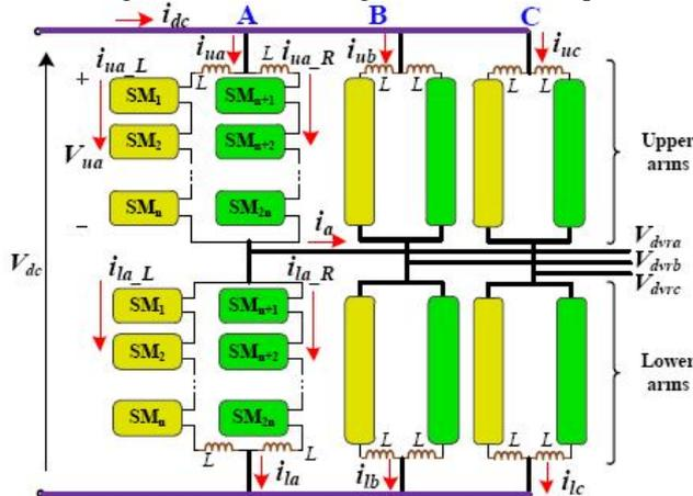
Fig 5: Three phase structure of parallel-DCM2C
