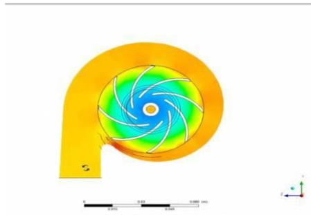
Fig 2 Maximum Total Pressure 137.7397 Pa. on impeller
