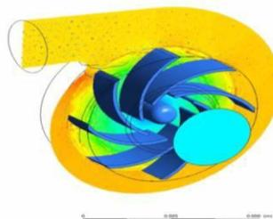
Fig 5 Velocity vector in Pump 0.548054 m/s
