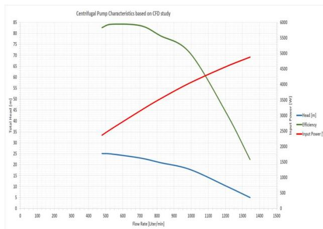
Fig 8 Graph shown in fig. centrifugal pump characteristics based on CFD.
