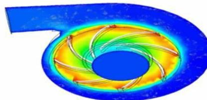
Fig 4 Velocity contour in Pump 0.548054 m/s
