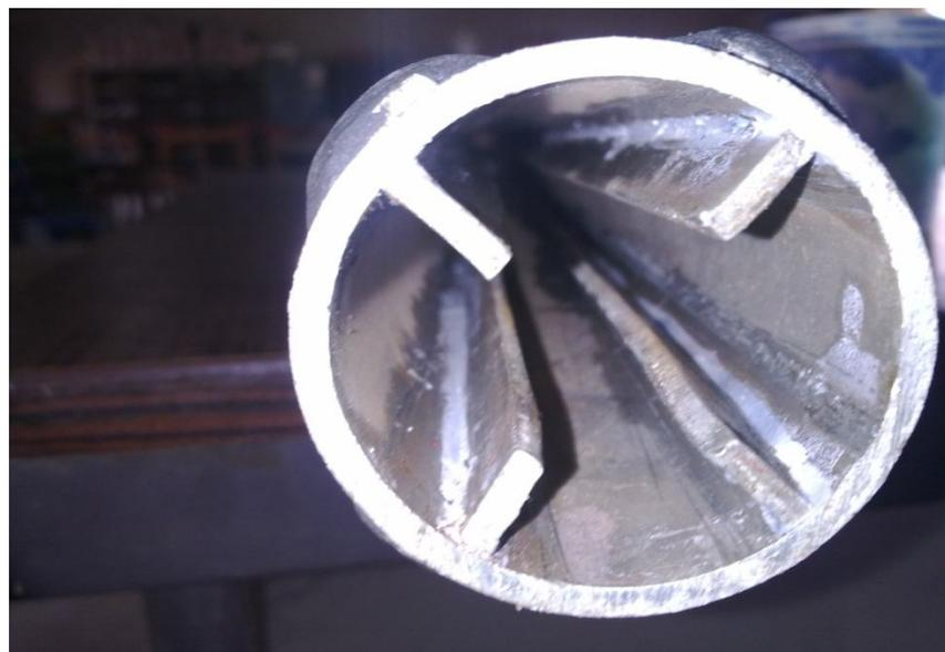
**Fig.3:** Internal fins on inner periphery of the tube
