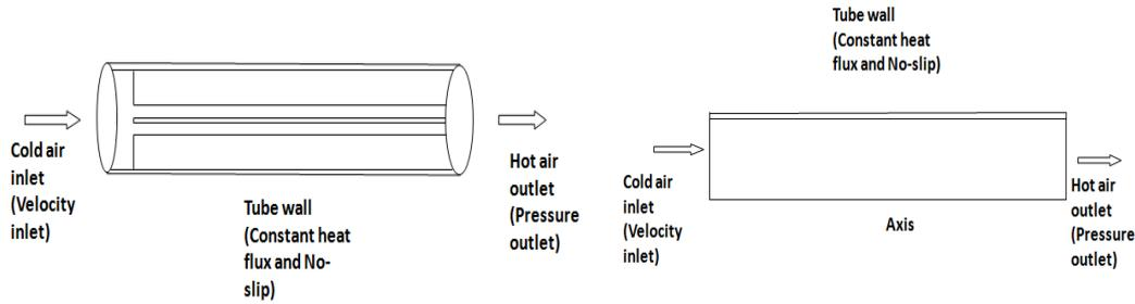
Fig. 4: Schematic diagram of computational domain and the boundary condition applied to it (a) finned tube; (b) unfinned tube
