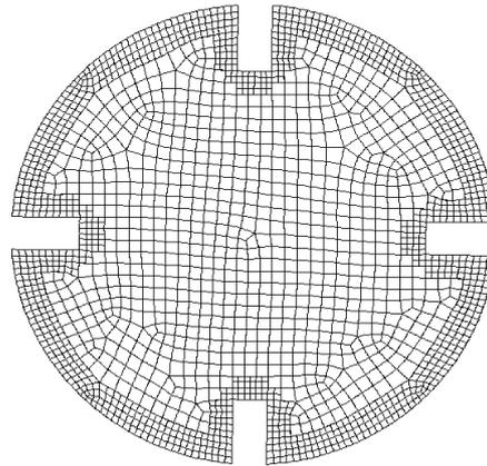
Fig.5: Cross sectional view of the internal finned tube showing the meshes inside the tube and around the fins
