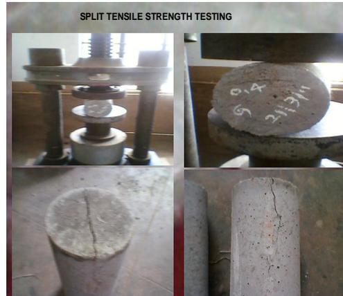
**Figure 2** Splitting tensile test
