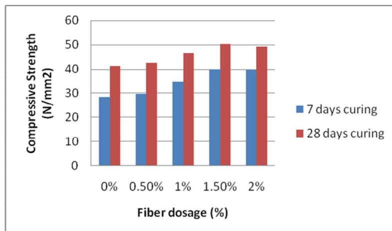
**Figure 3** Graphical Representations of Compressive Strength Test Results
