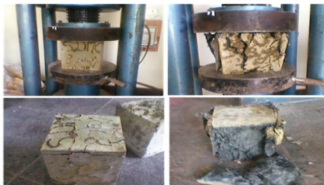
**Figure1** Compressive strength test
