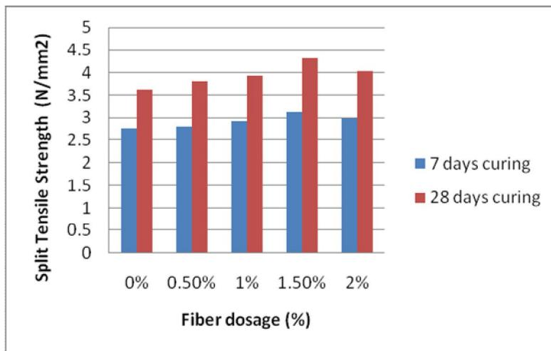
**Figure 4** Graphical Representation of Split Tensile Strength Test Results
