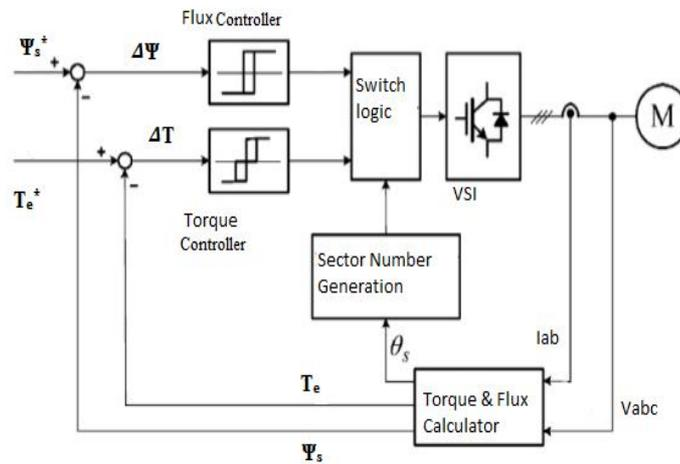
**Figure 1.**Block diagram of classical DTC method
