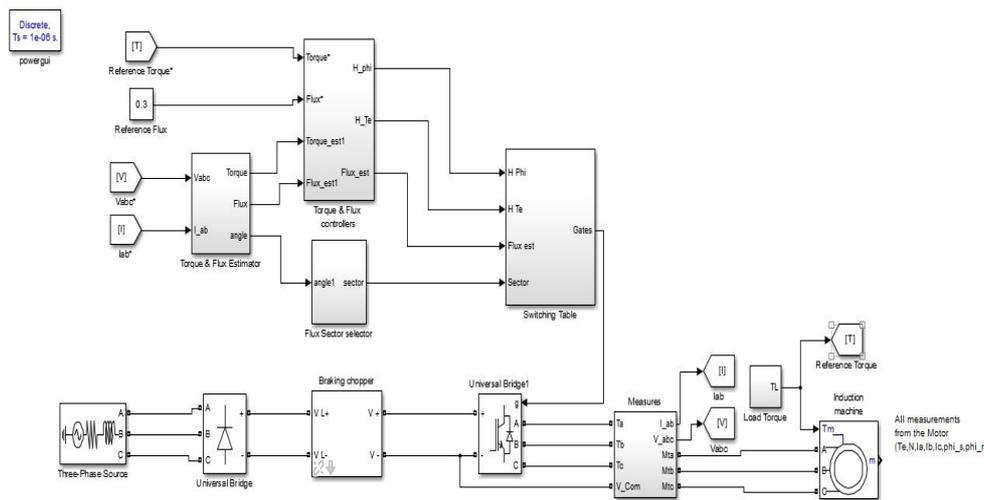
**Figure 4.** Block Diagram of MATLAB model for DTC drive
