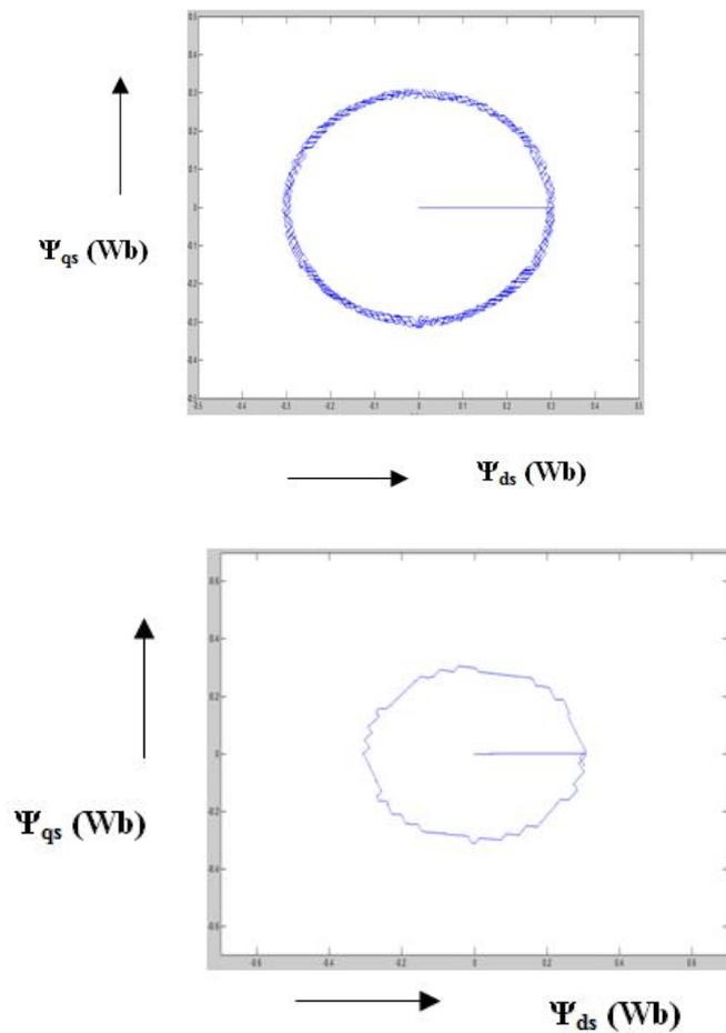
**Figure 6.** Stator flux (a) classical DTC (b) proposed DTC
