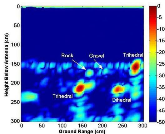
**Figure 2.** Laboratory Radar image of soil detailing the return of from the surface (150cm) and within the volume. The trihedral and dihedral are specially place reference targets.
