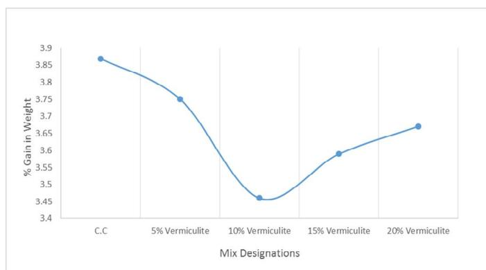
**Figure 1** Variation of Water Absorption for M30 and Vermiculite (5%, 10%, 15% & 20%)
