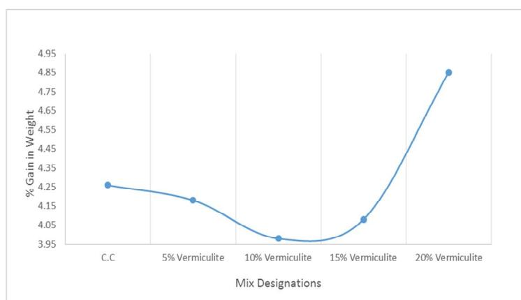
**Fig. 4.2** Variation of Water Absorption for M35 and Vermiculite (5%, 10%, 15% & 20%)
