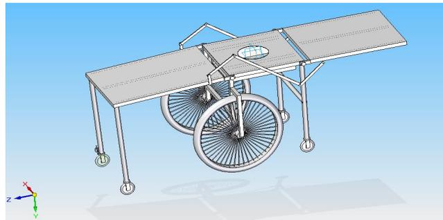
**Figure 4** 3D view of the device in stretcher position
