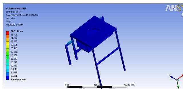
**Figure 5** Equivalent Von-Mises Stress Analysis result
