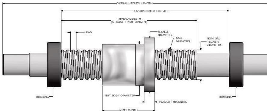
**Figure 1** Lead screw specification
