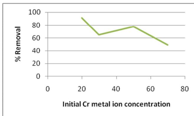
**Figure 6** Adsorption of Cr at various concentration levels
