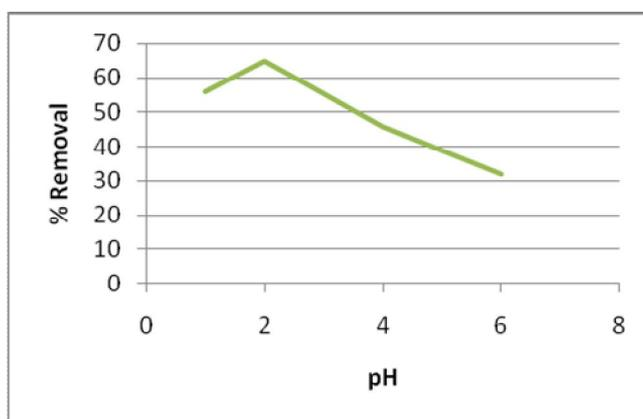
**Figure 4** Adsorption of Cr (VI) with increasing pH
