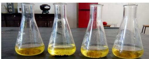
**Figure 2** Flasks containing chromium solution along with soapnut powder
