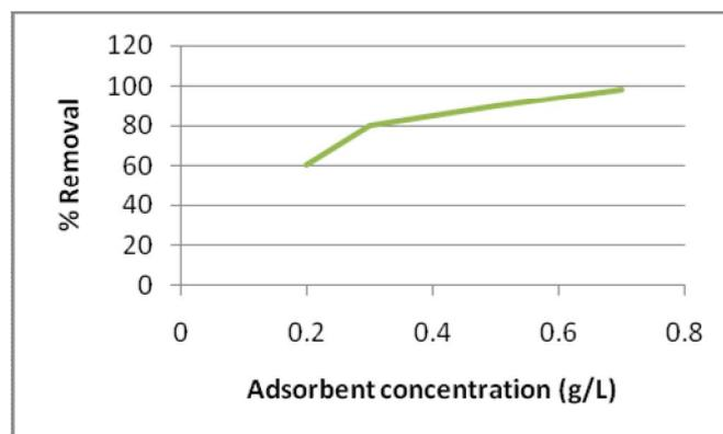
**Figure 7** Adsorption of Cr under varying adsorbent concentrations
