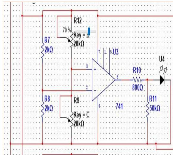
**Figure 10** Circuit diagram of LDR sensor
