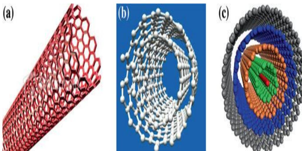
**Figure.2** Basic structures of a single-walled, b double- walled and c multi-walled carbon nano powder
