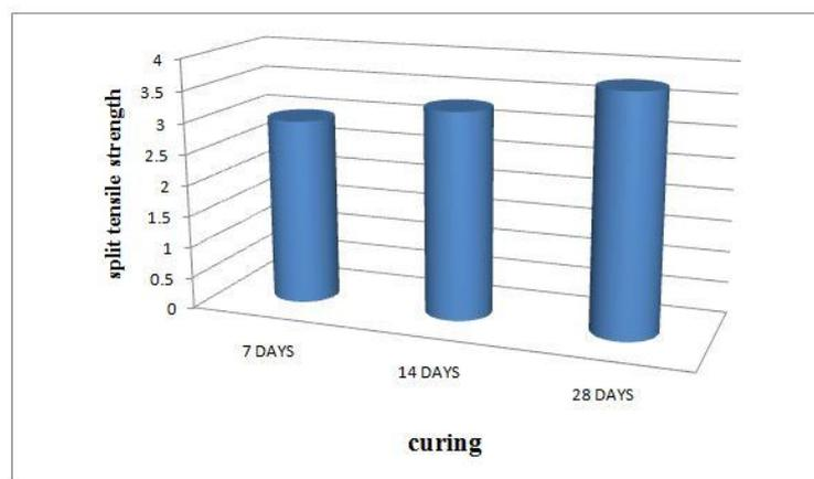
**Figure.4** Split Tensile Test Results
