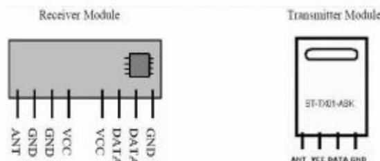
Figure 4. Radio Frequency module
