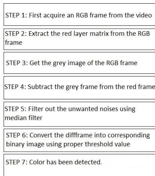
**Figure 2.** Flow of process for red color detection
