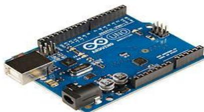
Figure 3. Arduino development board
