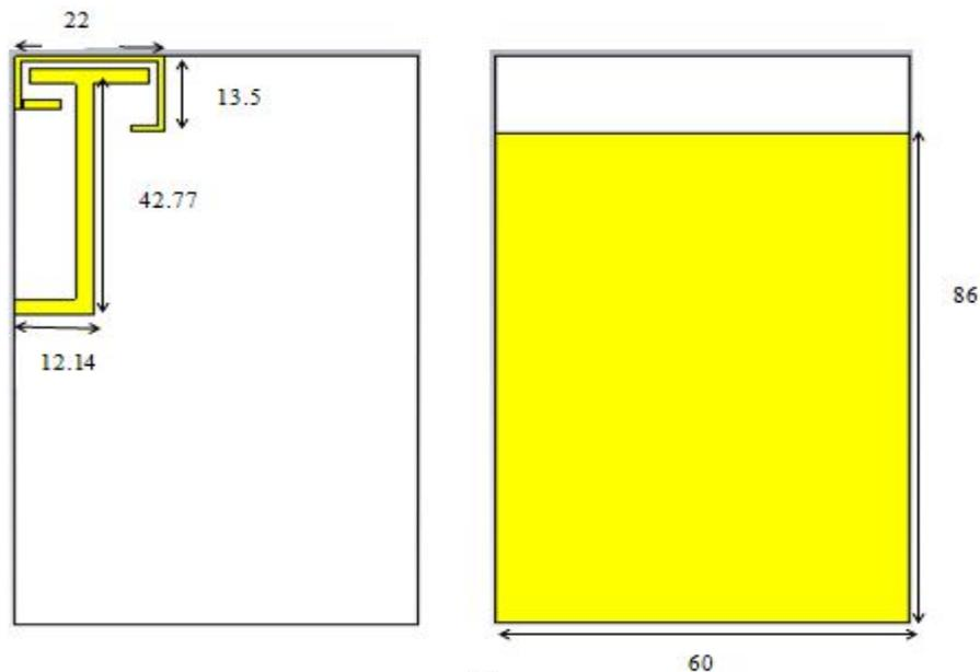
**Figure 1 - Simulated Design Of reconfigurable Antenna for Mobile Communication when diode is OFF (Top & Bottom View )**
