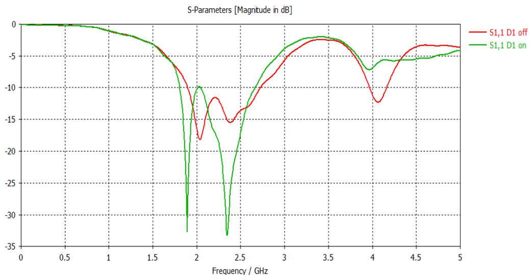
**Figure 5 - Return Loss In ON And OFF condition of PD1**
