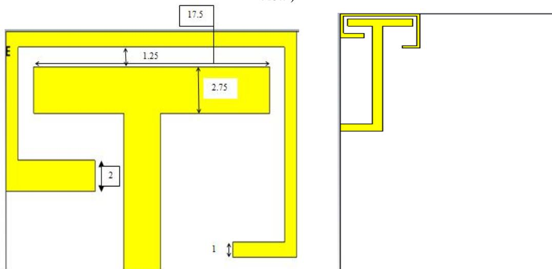
**Figure 2 - Simulated Design Of reconfigurable Antenna for Mobile Communication when diode is ON ( Top View ) with dimensions**
