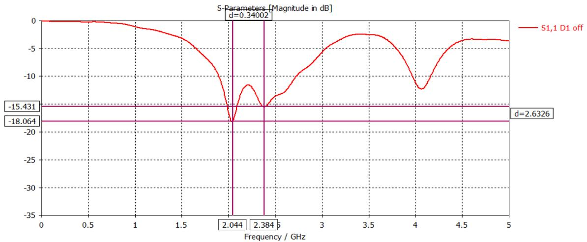
**Figure 3 - Return Loss Of Reconfigurable Antenna When PD1 OFF**
