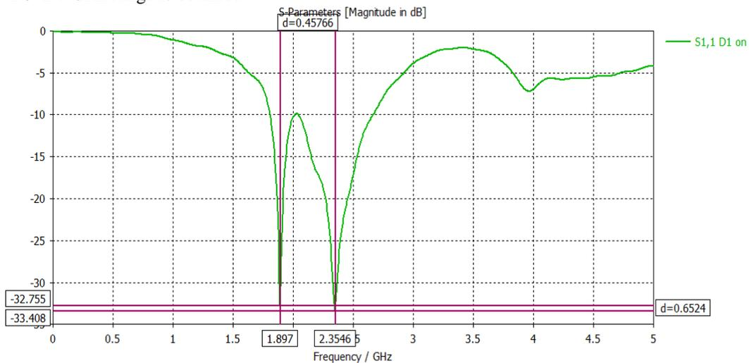
**Figure 4 - Return Loss Of Reconfigurable Antenna When PD1 ON**
