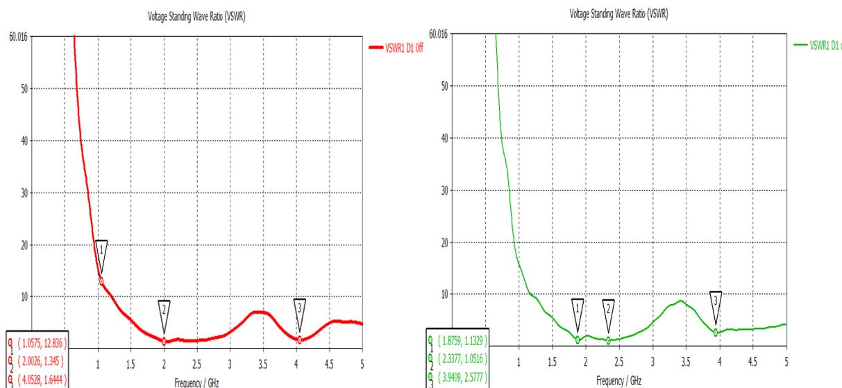
**Figure 6 - VSWR curve for case-I and case II of the proposed design**
