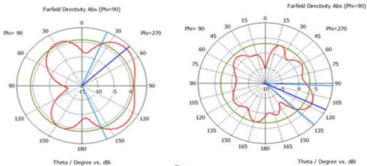
**Figure 7 -** Radiation patterns of the reconfigurable antenna for mobile communication at different frequencies
