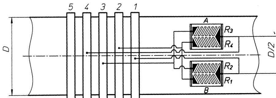
A B-measuring strain gages (rosettes for torsional deformation); 1, 2, 3, 4, 5-sliding rings
