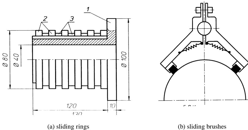
**Figure 3** Constructive view of the sliding rings and brushes
