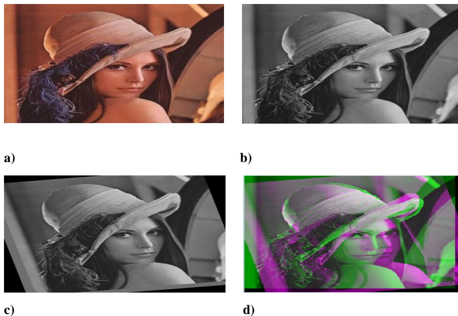
Fig 6: a) Reference Image b) Grayscale Image c) Sensed Image d) Registered Image
