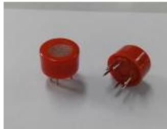
Fig 2.1.2.4. MQ3 Alcohol detection sensor
