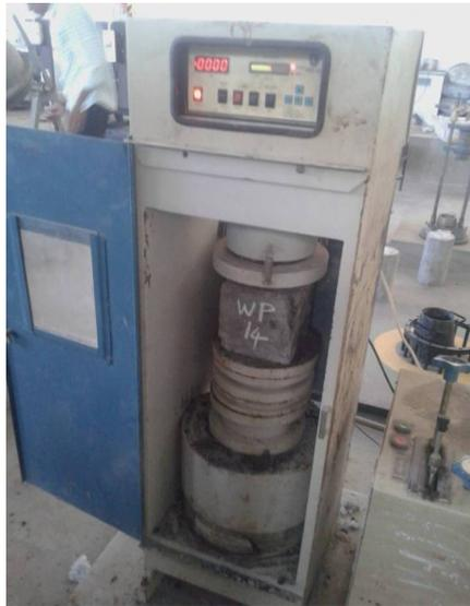
**Figure 3** Compression Strength Test For Cube
