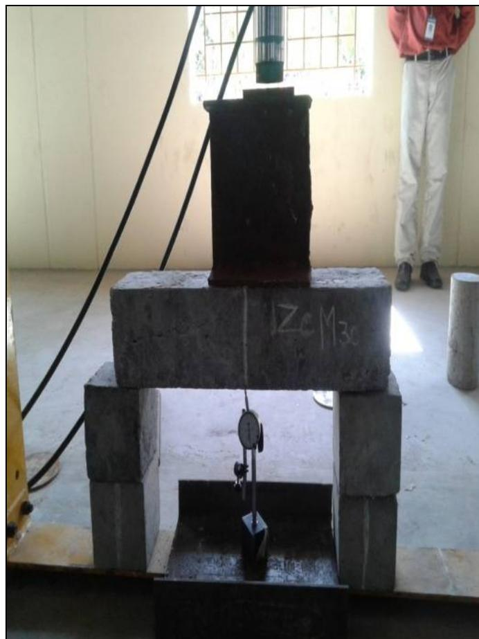
**Figure 5** Flexural Strength Testing Setup
