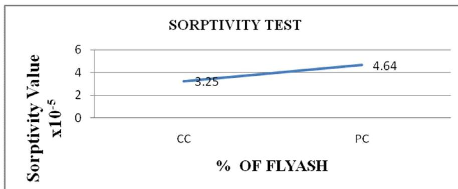
**Figure.7** Sorptivity Test Result on Cylinder
