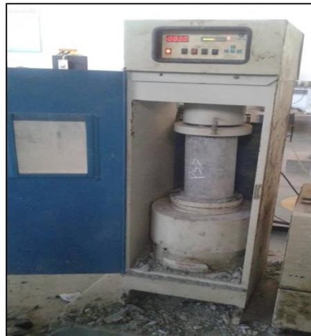
**Figure.4** Split Tensile Test Setup
