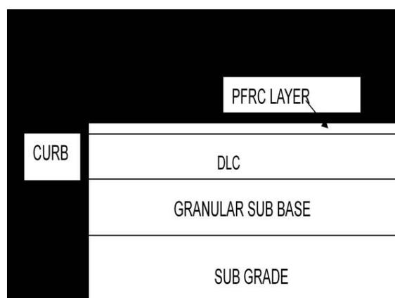
**Figure.2** Cross Section Of A Typical PFRC Pavement
