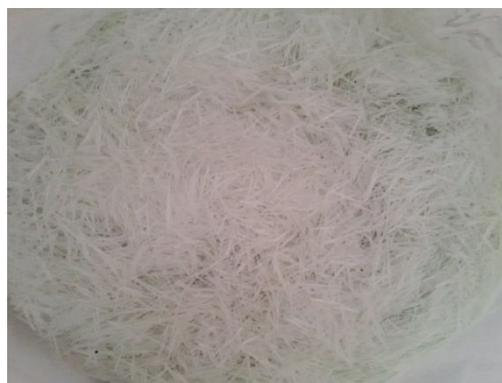
**Fig.1 AR Glass Fibre**
