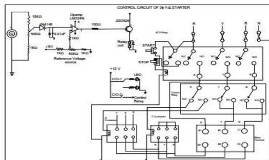
Figure 1 Circuit diagram of the starter.
