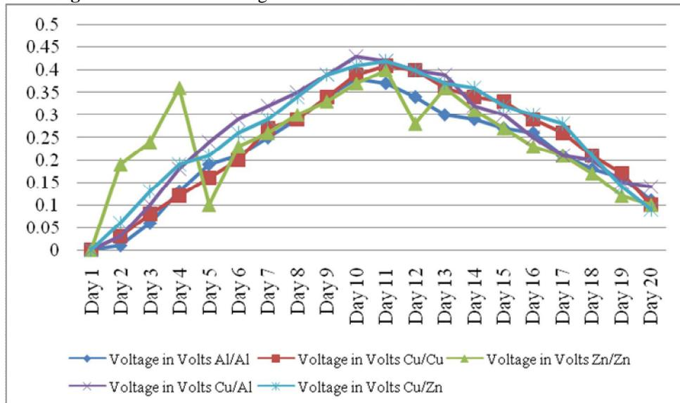
**Fig 6:** Generation of Voltage for Cow dung Based MFC before addition of Nutrients
