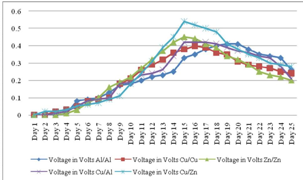
**Fig 4:** Generation of Voltage for Soil Based MFC before addition of Glucose
