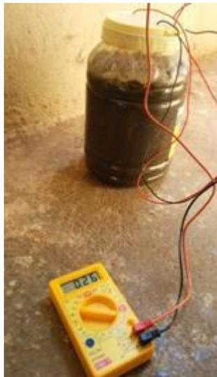
**Fig 1:** Model of soil based MFC
