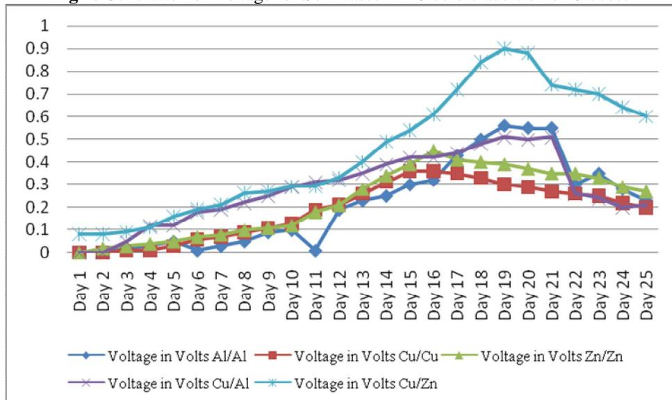
**Fig 5:** Generation of Voltage for Soil Based MFC after addition of Nutrients
