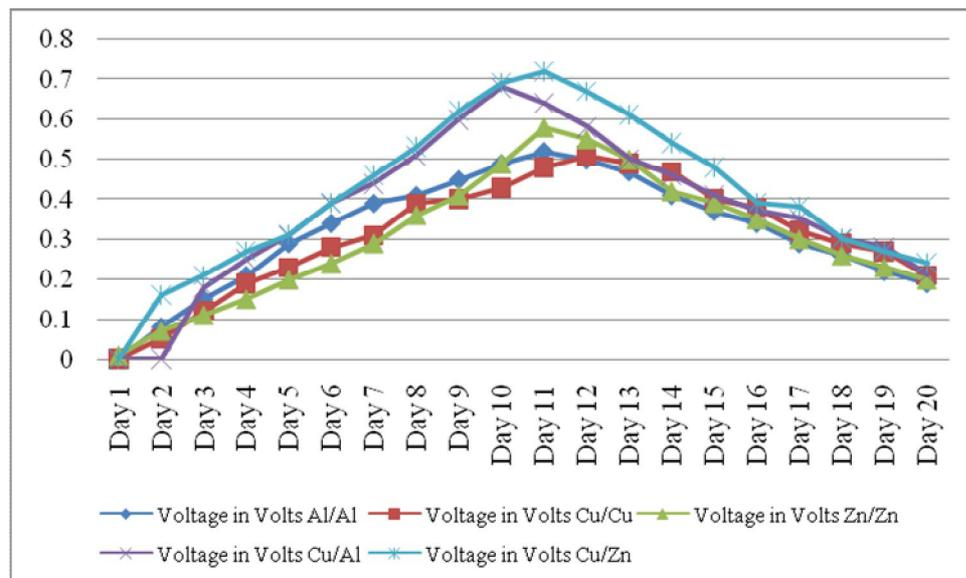
**Fig 7:** Generation of Voltage for Cow Dung Based MFC After addition of Nutrients
