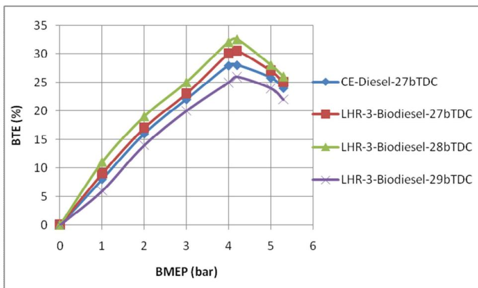
**Figure.4.** Variation of brake thermal efficiency (BTE) with brake mean effective pressure (BMEP) in engine with LHR combustion chamber with biodiesel at various injection timings at an injector opening pressure of 190 bar.
