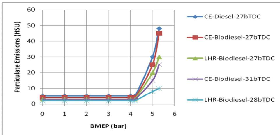
**Figure.5** Variation of particulate emissions with biodiesel operation on both versions of the engine at recommended injection timing and optimum injection timing.
