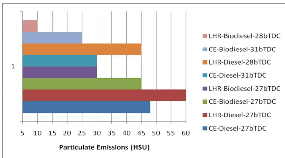
**Figure.6.** Bar charts showing the variation of particulate emissions at full load operation with test fuels with conventional engine (CE) and engine with LHR combustion chamber at recommended and optimized injection timings at an injector opening pressure of 190 bar.
