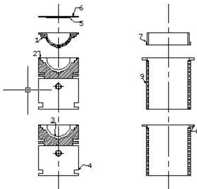
1.Supe 1. Piston crown with threads, 2. Superni gasket, 3. Air gap in piston, 4. Body of piston, 5. Ceramic coating on inside portion of cylinder head, 6. Cylinder head, 7.Superni insert with threads, 8.Air gap in liner, 9.Liner
