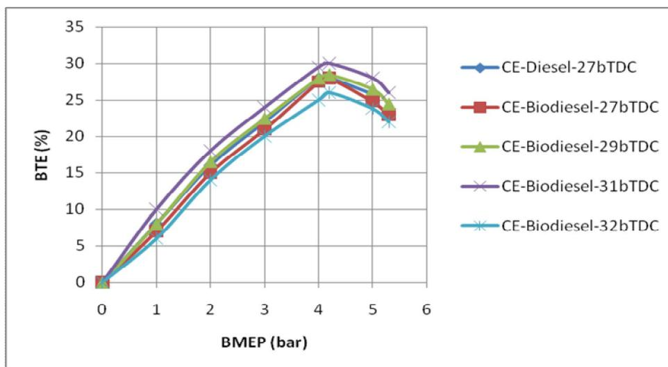
**Figure. 3** Variation of brake thermal efficiency (BTE) with brake mean effective pressure (BMEP) in conventional engine (CE) with biodiesel at various injection timings at an injector opening pressure of 190 bar.
