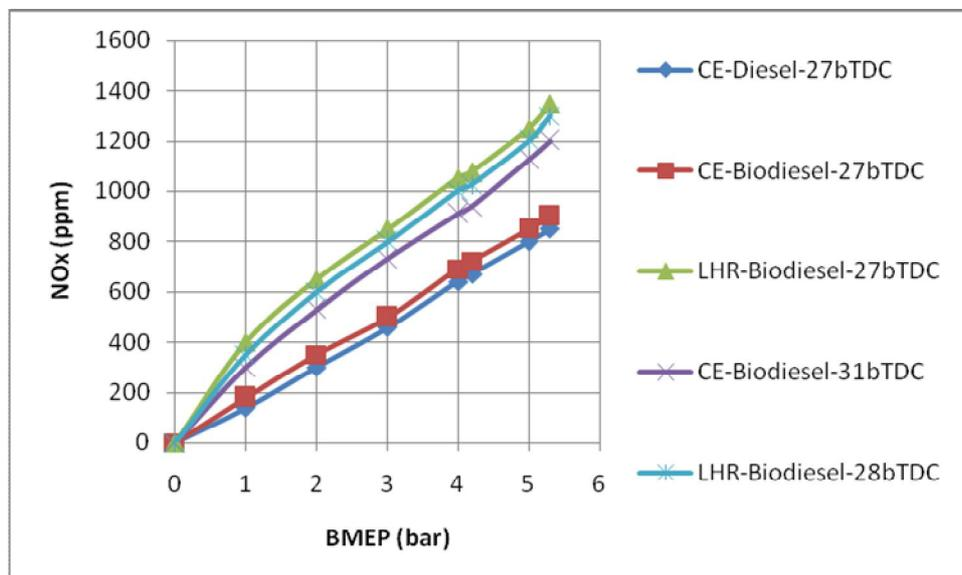
**Figure.7.** Variation of nitrogen oxide levels with biodiesel operation on both versions of the engine at recommended injection timing and optimum injection timing.
