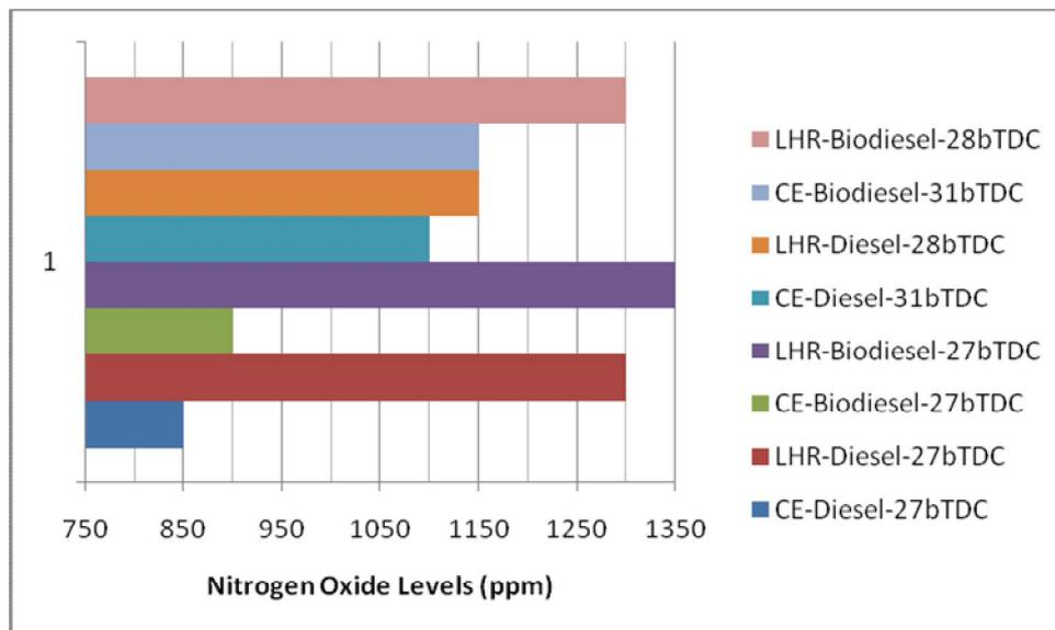
**Figure.8.** Bar charts showing the variation of nitrogen oxide levels at full load operation with test fuels with conventional engine (CE) and engine with LHR combustion chamber at recommended and optimized injection timings at an injector opening pressure of 190 bar.
