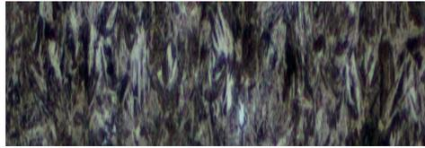
**Figure 3(d)** consists of martensite structure (20°C/Sec) corresponds to a smaller number of crystals with granular morphology in the structure.
