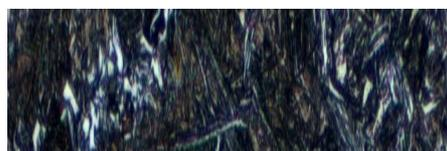
**Figure 3(b)** Bainite phase formed ( $5^{\circ}\text{C}/\text{sec}$ ) consists of feathery needle like structure of upper or lower bainite formed.
