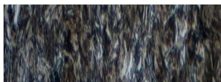
**Figure 3(c)** consists of bainite (the light crystals) ( $8^{\circ}\text{C}/\text{sec}$ ) and martensite (the dark crystals) formed in the stage.
