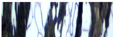
**Figure3(a)** it consists of ferrite and pearlite forms due to lower cooling rate  $5^{\circ}\text{C}/\text{sec}$ .
