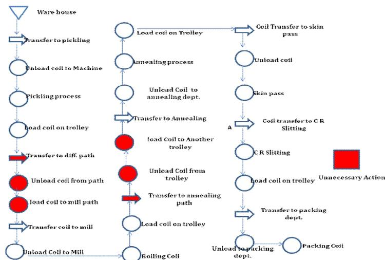
**Figure 24:** Existing flow process chart
