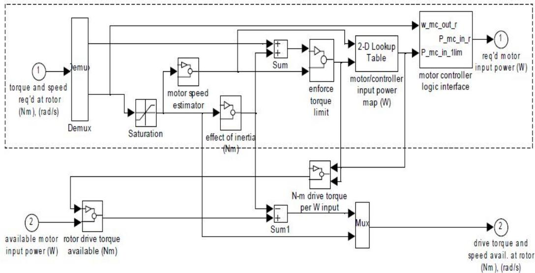
**Figure 4:** Motor/ Controller Simulink Block model
