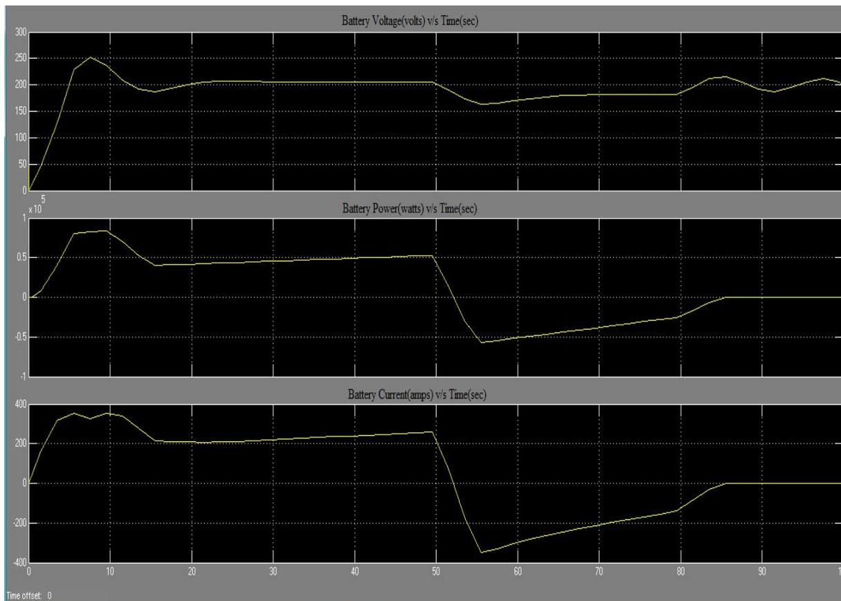
Figure 7: Battery voltage, Power and current for Indian Highway Drive cycle.
