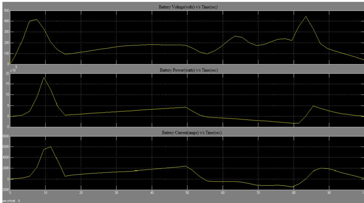
**Figure 8:** Battery Voltage, Current and Power for Indian Urban Drive cycle.
