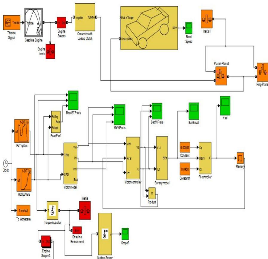
**Figure 1: Simulink model of Hybrid Electric Vehicle (HEV)**
