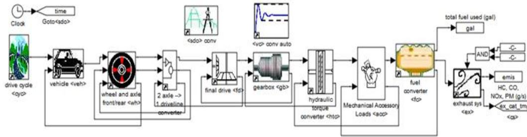
Figure 2: Simulink model of a Conventional Vehicle
