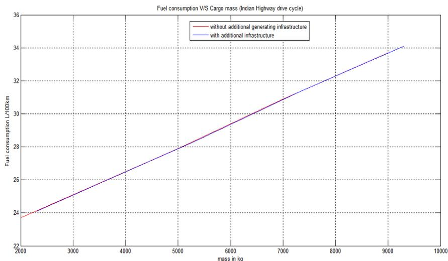
Figure 11 : Effect on fuel consumption with/without generating infrastructure (Indian Highway drive cycle)
