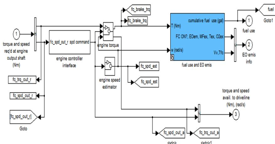
Figure 3: Engine block of Conventional vehicle Modeled in MATLAB/Simulink
