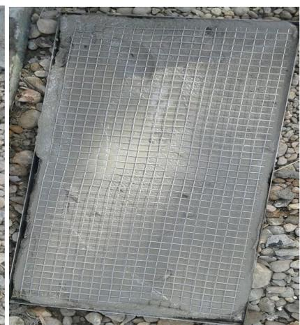
**Figure.7.**Finishing stage of steel mesh with 15% industrial waste, P.V.C coated mesh with 600 x 300 mm slab size and Steel mesh with 600 x 300 mm slab size
