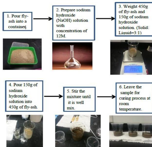
**Figure. 8** Preparation Of Geo Polymer Sample
