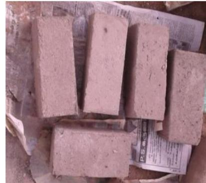
**Figure. 12** Geopolymer Bricks
