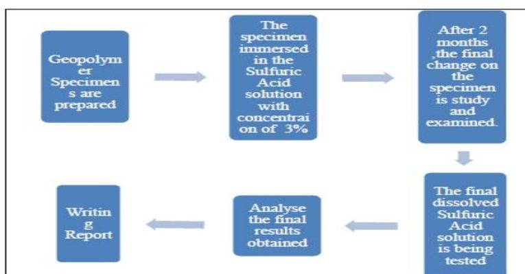
Figure.7. Test On Sulfuric Acid Resistance
