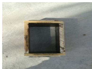
**Figure. 10** Brick Mould
