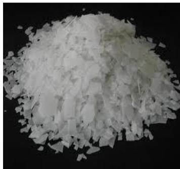
**Figure. 2** NaOH – Flakes
