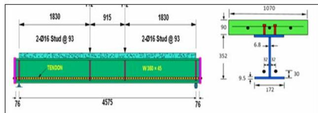
**Figure.2** Details of Beam (VS-2)
