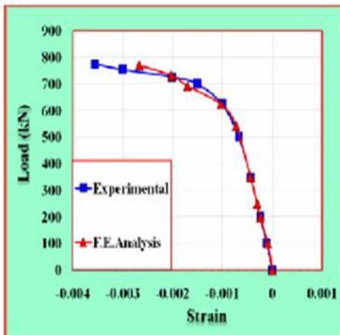
Figure.21 Load-strain curve for extreme compression concrete fiber for VS-3
