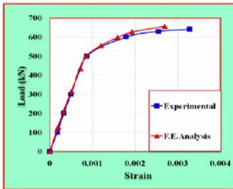
Figure.13 Load-strain curve for extreme compression concrete fiber of vs-1
