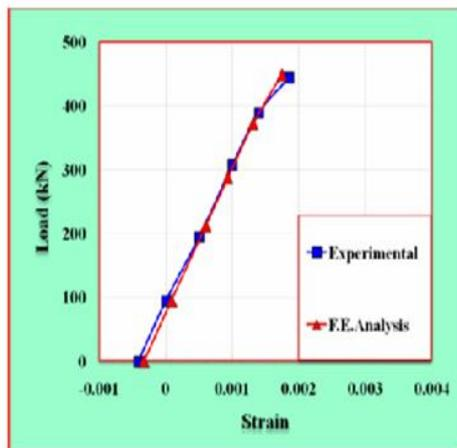
Figure.15 Load-strain curve for bottom flange for VS-1
