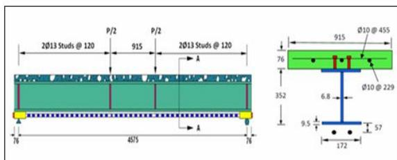
**Figure.1** Details of Beam (VS-1)
