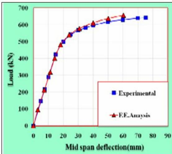
**Figure.4** Load-Deflection Curve for Beam VS-1
