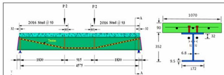
**Figure. 3** Details of Beam (VS-3)
