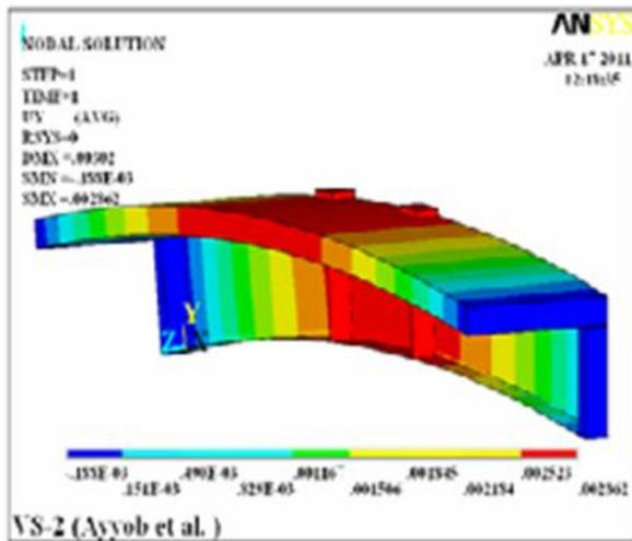
Figure.9 Initial Camber of the Beam VS-2 With no Applied Concentrated Load
