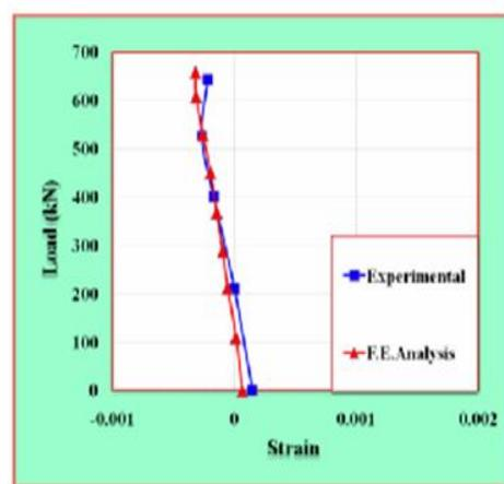
Figure.16 Load-strain curve for top flange for VS-1
