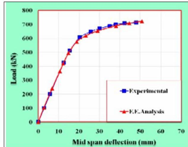
**Figure.5.** Load-Deflection Curve for Beam VS-2
