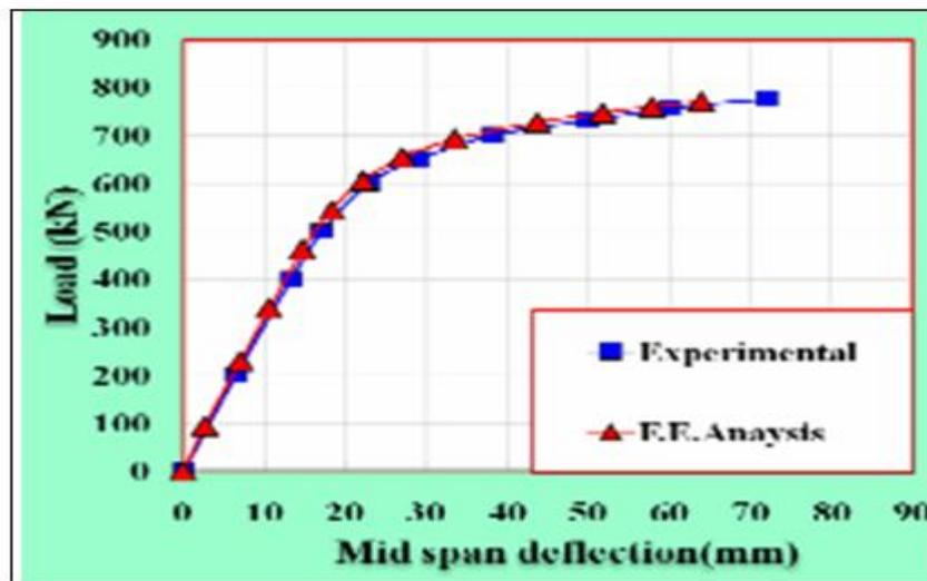
**Figure.6** Load-Deflection Curve for Beam VS-3
