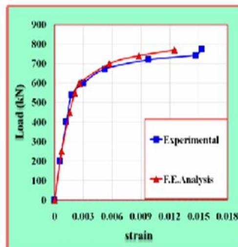
Figure. 24 Load-strain curve for bottom flange for VS-3
