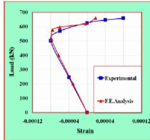
Figure 18 Load-strain curve for bottom concrete fiber for VS-2.
