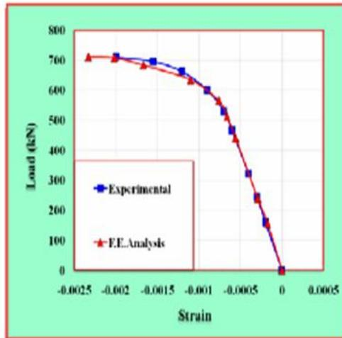
Figure 17 Load-strain curve for extreme compression concrete fiber of VS-2.
