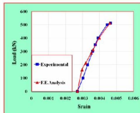
Figure.14 Load-strain curve for prestressed bars for VS-1
