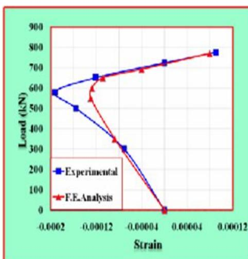
Figure.23 Load-strain curve for top flange for VS-3
