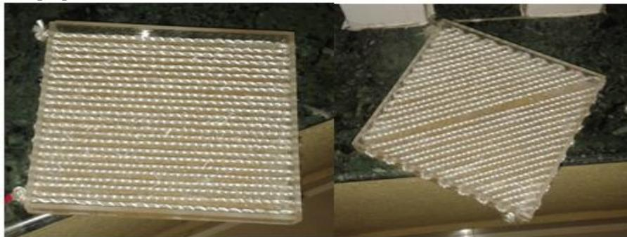
**Fig 5.1** Acrylic Moulds with woven glass fiber
