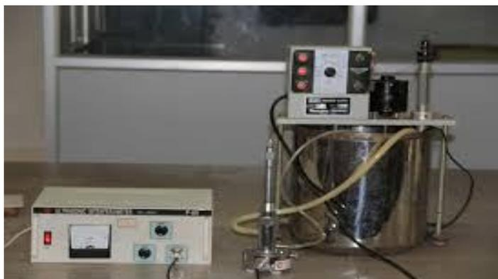
Figure 1 Thermostated Ultrasonic Interferometer equipment
