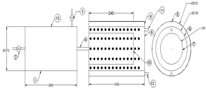
**Figure.2.** Details of catalytic converter.
