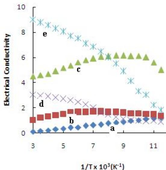
**Fig.1.** Electrical conductivity v/s inverse temperature of as deposited  $CdS_xSe_{1-x}$  thin films of composition parameter a)  $x=0$  b)  $x=0.25$  c)  $x=0.5$  d)  $x=.75$  e)  $x=1.0$
