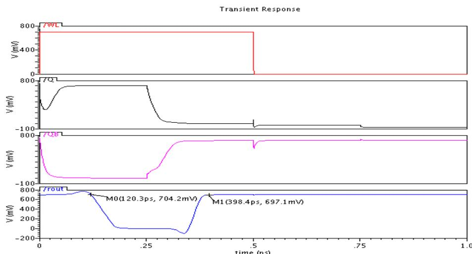
**Fig 11:** The waveform of read operation in FinFET based 7T SRAM cell.
