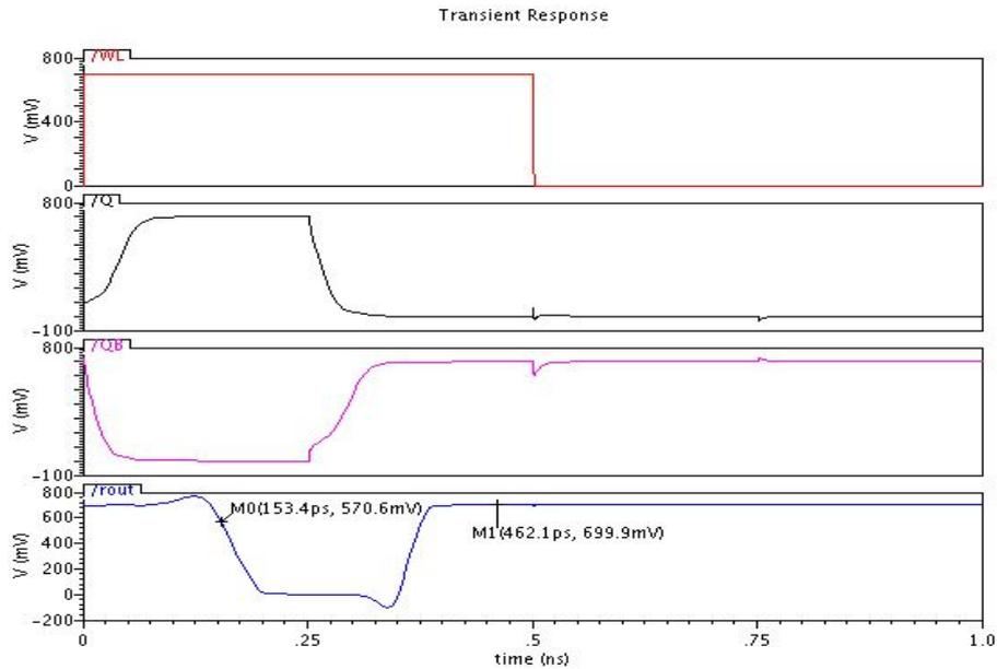
**Fig 7:** The waveform of read operation in FinFET based 6T SRAM cell.
