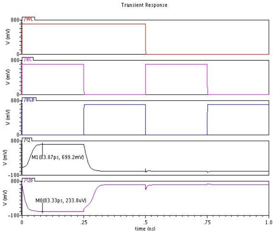
Fig 6: The waveform of write operation in FinFET based 6T SRAM cell.
