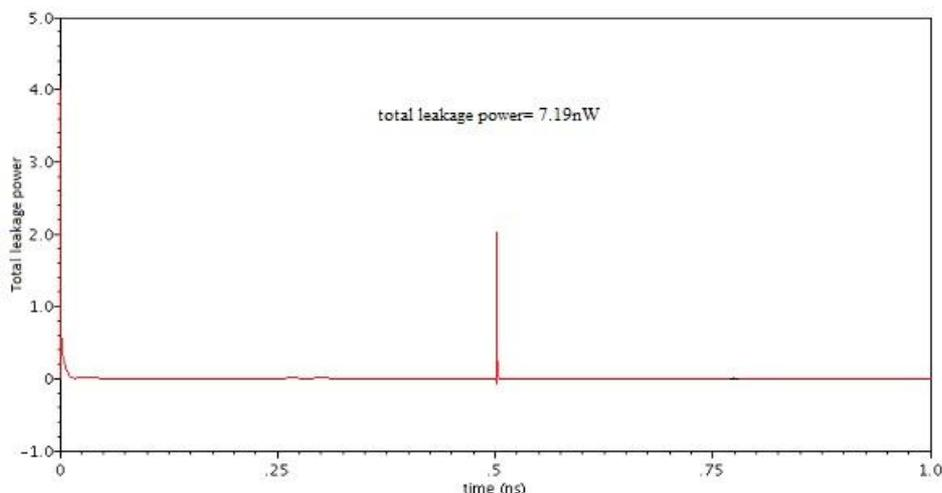
**Fig 13:** The waveform of total leakage power in FinFET based 7T SRAM cell.
