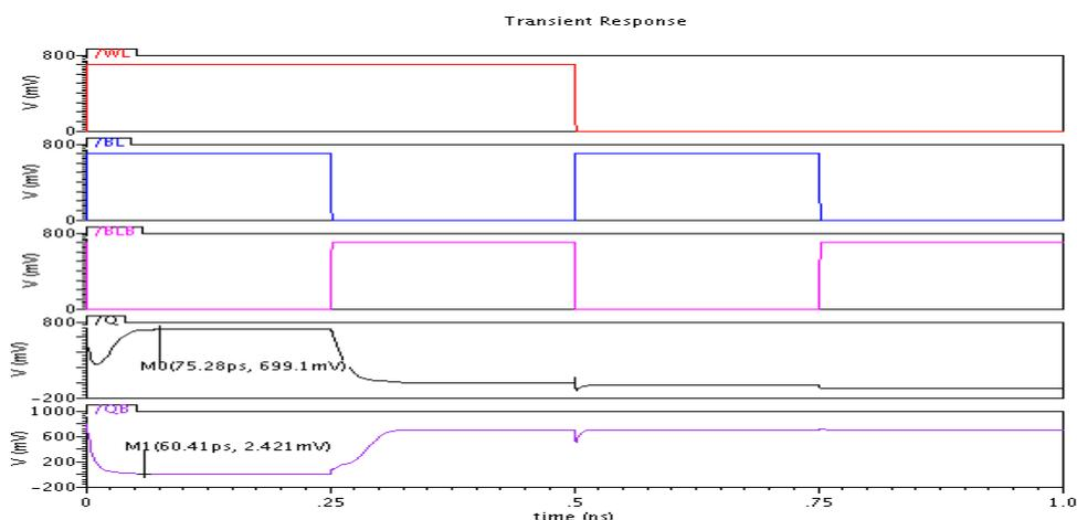
**Fig 10:** The waveform of write operation in FinFET based 7T SRAM cell.
