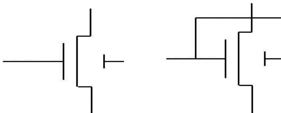
**Figure 2:** Independent Gate and Short Gate FinFET
