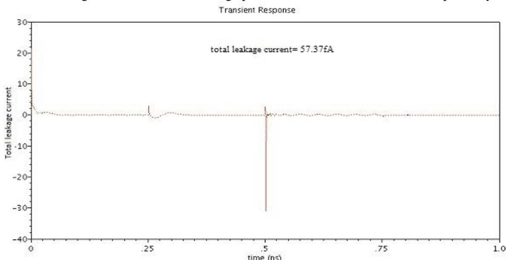
**Fig 12:** The waveform of total leakage current in FinFET based 7T SRAM cell.
