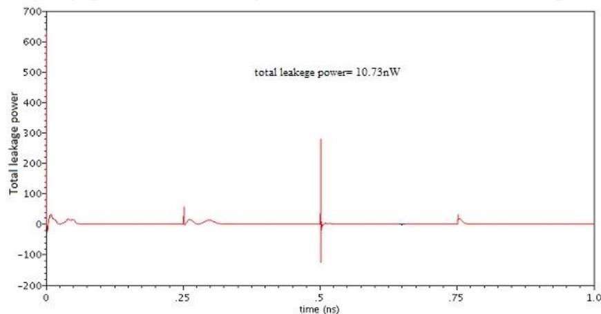
**Fig 8:** The waveform of total leakage power in 6T FinFET SRAM cell.
