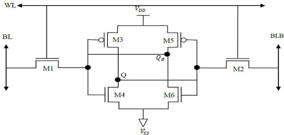
**Fig 3:** Conventional 6T SRAM Cell
