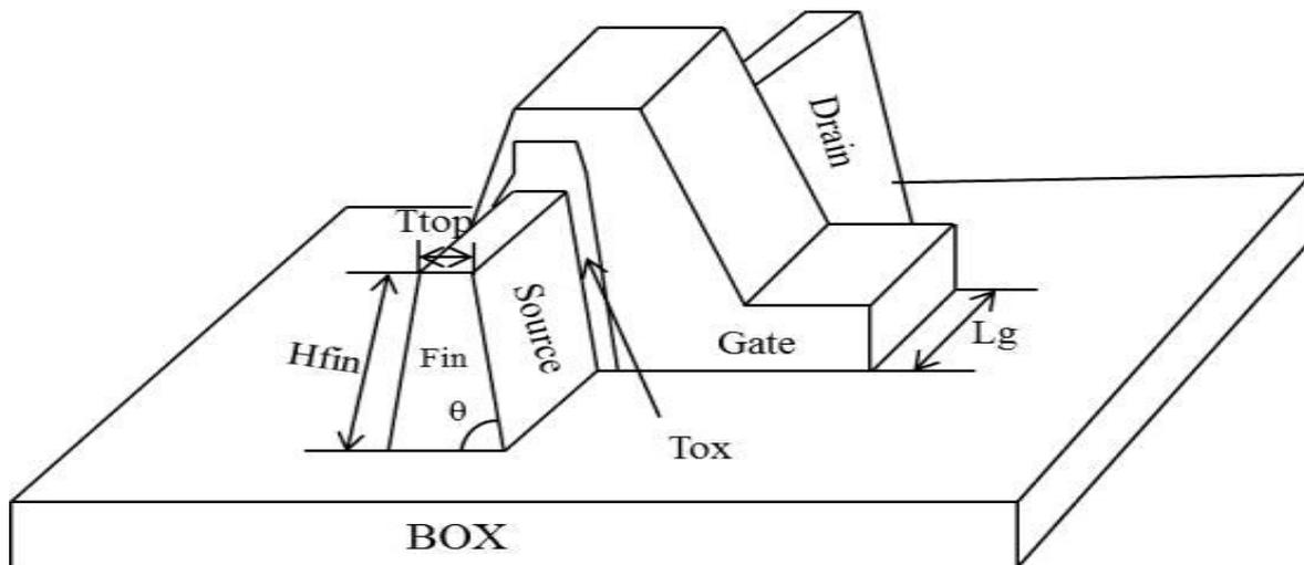
**Figure 1:** 3D geometry of FinFET
