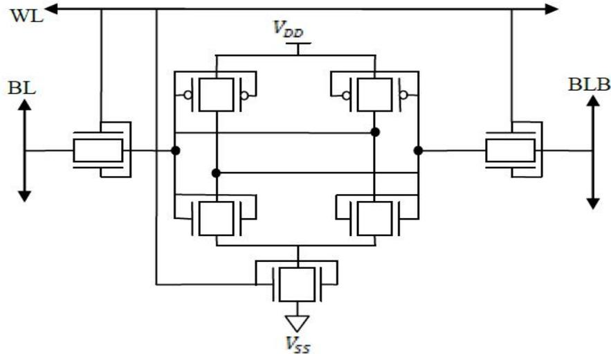
Fig 5 FinFET based proposed 7T SRAM cell
