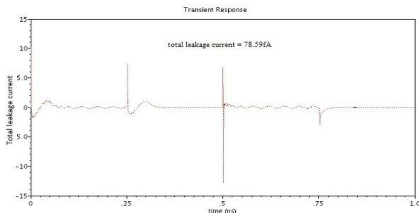
**Fig 9:** The waveform of total leakage current in FinFET based 6T SRAM cell.
