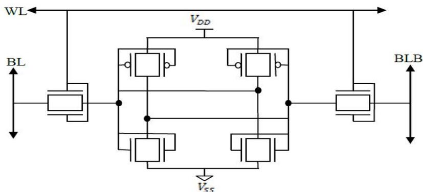
**Fig 4** FinFET based 6T SRAM cell
