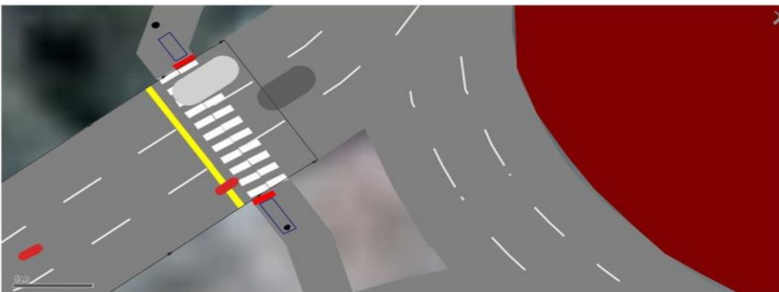
**Figure 7:** Traffic signal changes automatically when pedestrian signal detects the pedestrian
