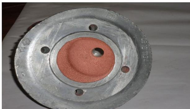
**Plate 1** Photographic view of copper coated cylinder head
