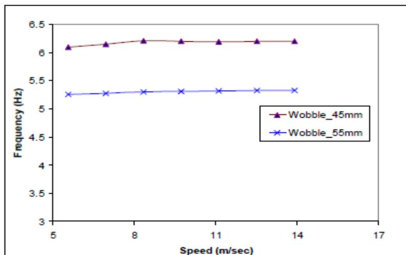
**Figure 3:** Variation of Wobble mode frequency (for 45 mm and 55 mm steering offset) with speed.
