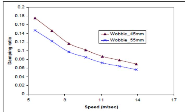
**Figure 4:** Variation of Wobble mode damping ratio (for 45 mm and 55 mm steering offset) with speed.
