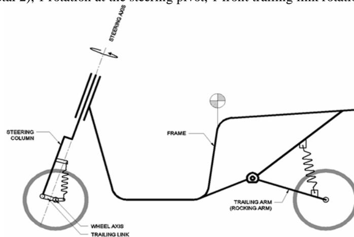
**Figure 1:** A schematic of a three wheeled vehicle. [1]
