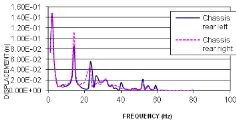
**Figure 5:** Variation in displacement at the left and right end of the rear chassis
