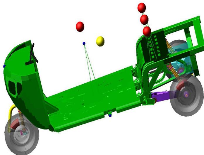
**Figure 2:** Multi-body dynamic model of a three wheeler. In this figure D, P1, P2, P3 and O represent the CG location of the driver, three passengers and the chassis.
