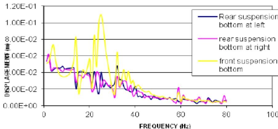
**Figure 6:** Variation in the displacement values at the suspension bottoms
