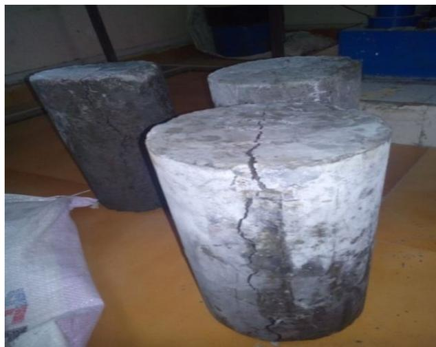
**Image3:** Failure Pattern of Concrete cylinder
