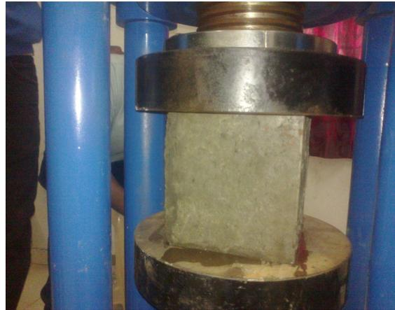
**Image1:** Compressive Testing of Concrete Block
