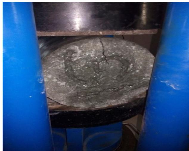
**Image2:** Split tensile Testing of Concrete cylinder
