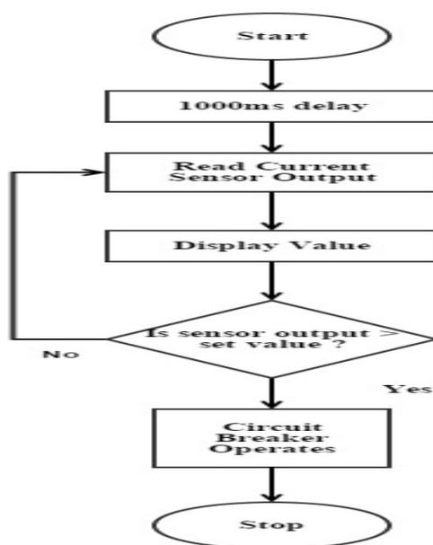
**Figure 2** Flowchart (Program Logic)
