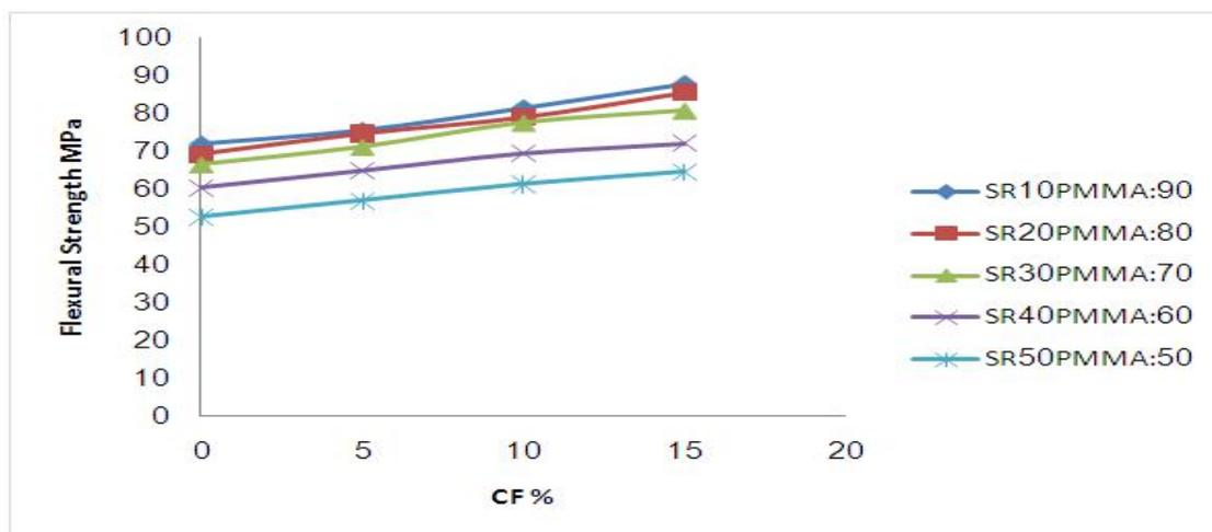
**Fig.4** Effect CF on the Flexural Strength PMMA:SR Polymer Blends
