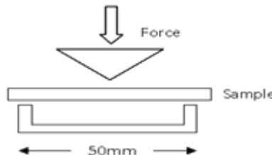
**Fig.2** Schematic illustration of flexural strength test arrangement
