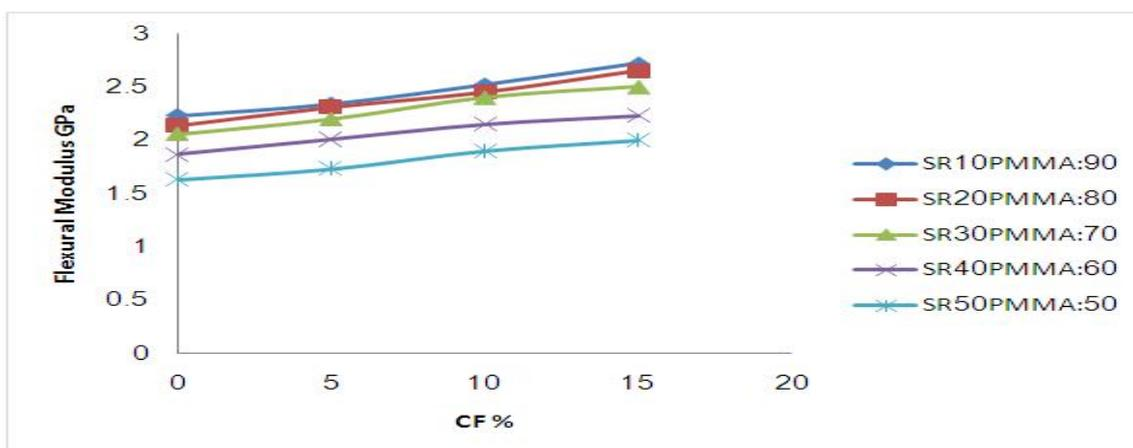
**Fig.5** Effect CF on the Flexural Modulus of PMMA:SR Polymer Blends
