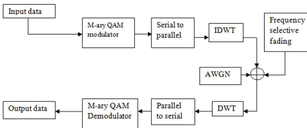
**Figure 4** WPM based mobile communication model
