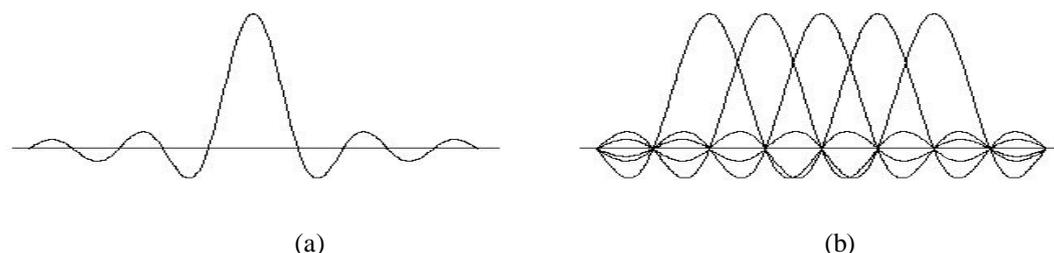
**Figure 1** Spectrum of (a) OFDM sub channel (b) OFDM channel
