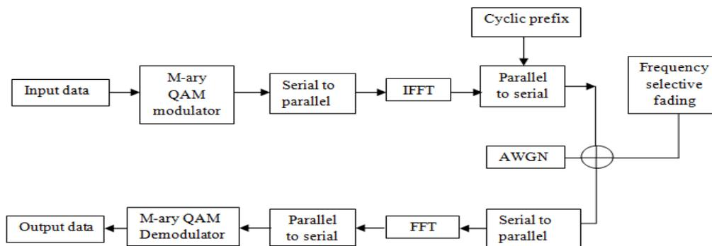
**Figure 3** OFDM based mobile communication model
