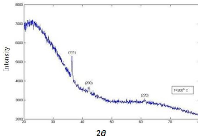
**Figure 1:** XRD reflection peaks of Cu<sub>2</sub>O thin film synthesized by CVD route.
