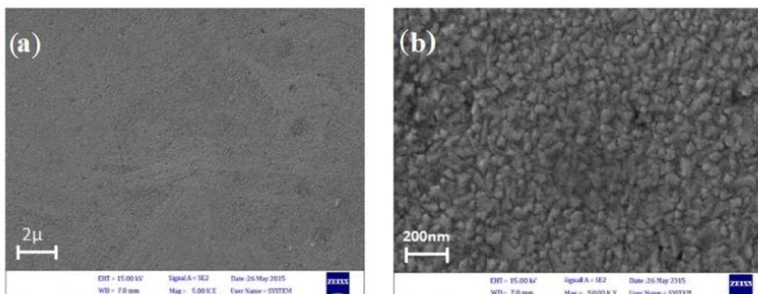
**Figure 3:** FE-SEM micrograph of Cu<sub>2</sub>O thin film deposited at 200 °C by CVD route, magnified for a) 2µm b) 200nm.
