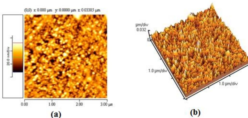
**Figure 5:** 2D and 3D AFM image of  $\text{Cu}_2\text{O}$  thin film synthesized at  $200^\circ\text{C}$ .
