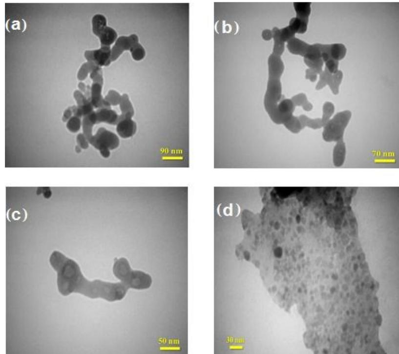
**Figure 6:** Different TEM images of  $\text{Cu}_2\text{O}$  synthesized at  $200^\circ\text{C}$ .
