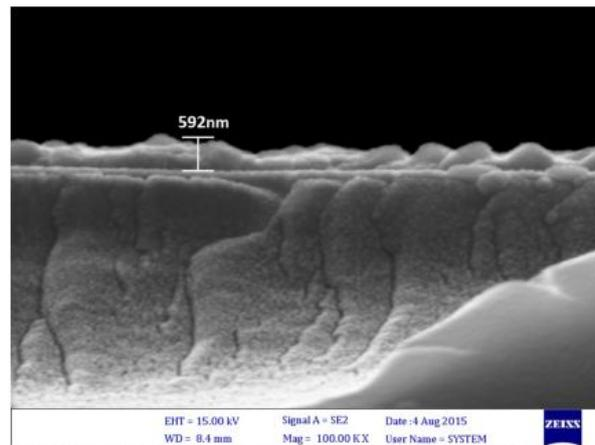
**Figure 4:** Thickness of  $\text{Cu}_2\text{O}$  thin films measured by SEM cross section resulted of 59.2 nm.
