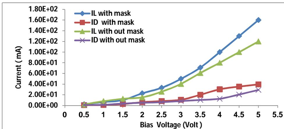
Figure 9 I-V characteristics of the MWCNTs-PSi IR detector fabricated with and without aluminum mask.
