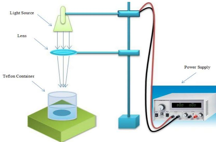
**Figure 1** The set up of the photochemical etching process.
