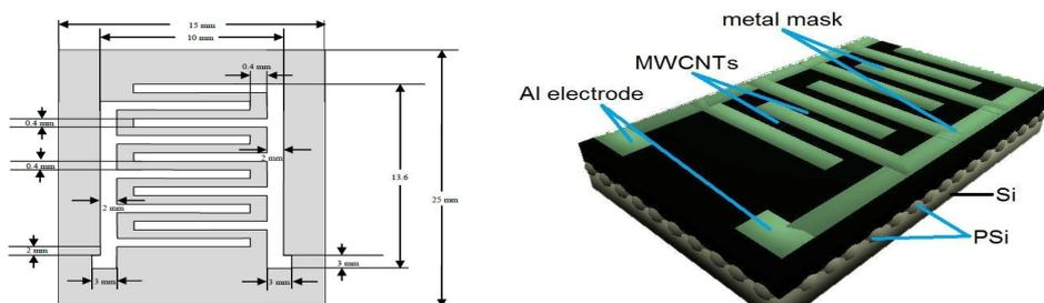
**Figure3** (a) Schematic diagram of the IDE masks utilized in this work, (b) Final shape for the fabricated photoconductive detector.
