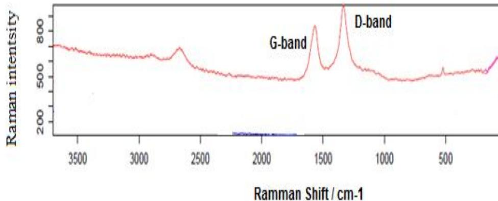
**Figure 7** Raman spectrum the MWCNTs deposited on PSi nanosurface.
