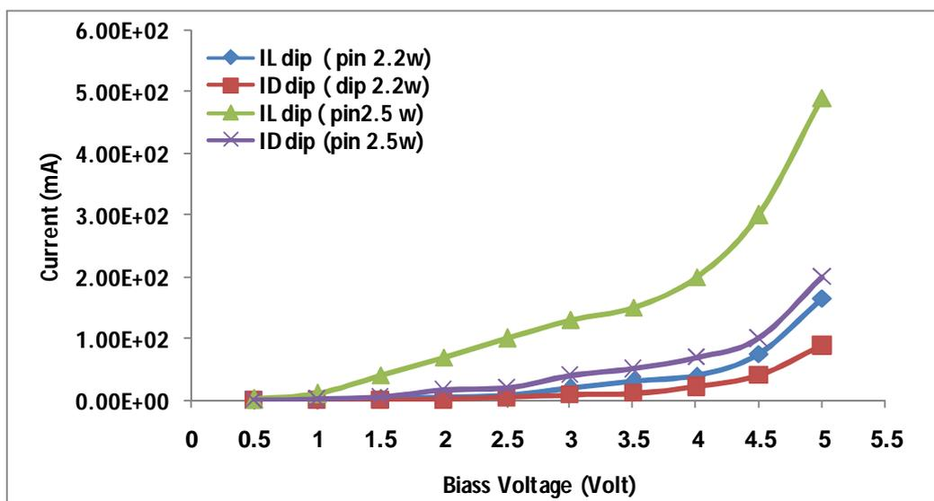
**Figure8** I-V characteristics of the MWCNTs-PSi IR detector (a) P<sub>in</sub> 2.2W,(b) P<sub>in</sub> 2.5W. IL is the photo current and ID is the dark current.
