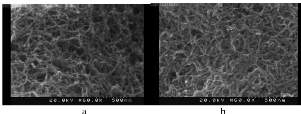
**Figure 6:** SEM images for the MWCNTs deposited on PSi nanosurface by:
