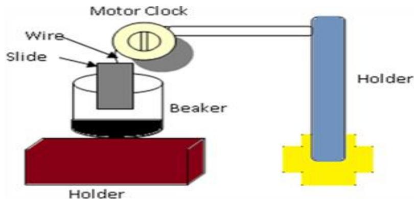
**Figure 2** Schematic diagram of simple dip coating system.
