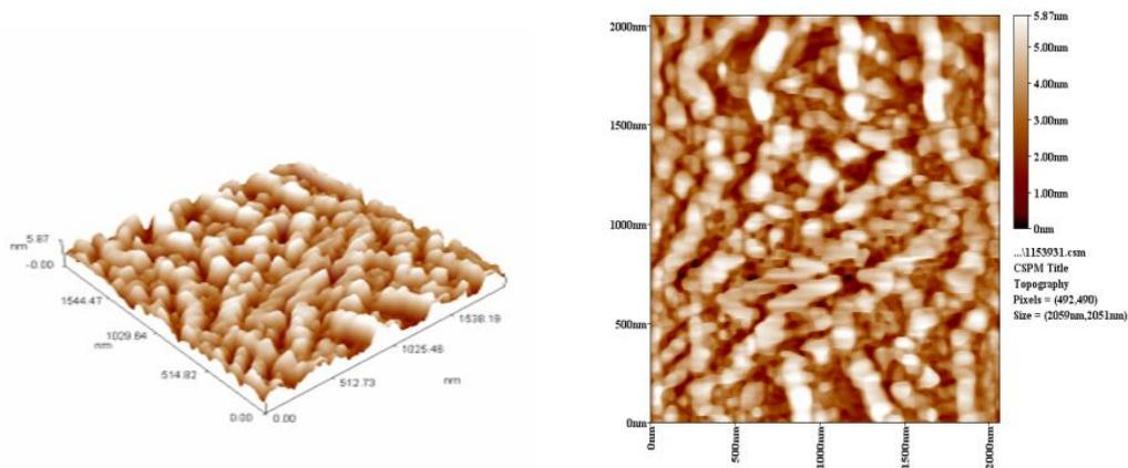
**Figure 5** AFM images for the MWCNTs deposited on PSi nanosurface
