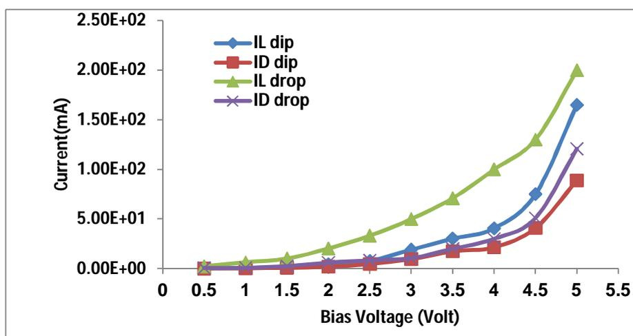
Figure 10 I-V characteristics of the MWCNTs-PSi IR detector fabricated by dip and drop methods for the deposited film
