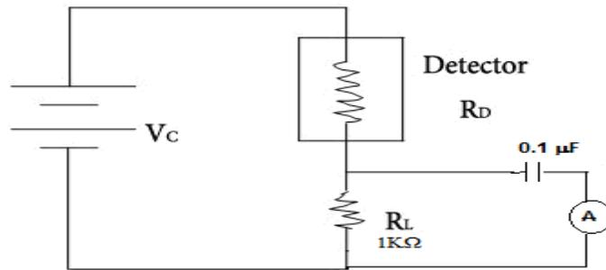
**Figure 4** The operation circuit diagram of Infrared photoconductive detector.
