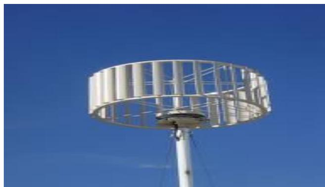
**Fig 2.2:** Vertical -Axis Wind Turbine
