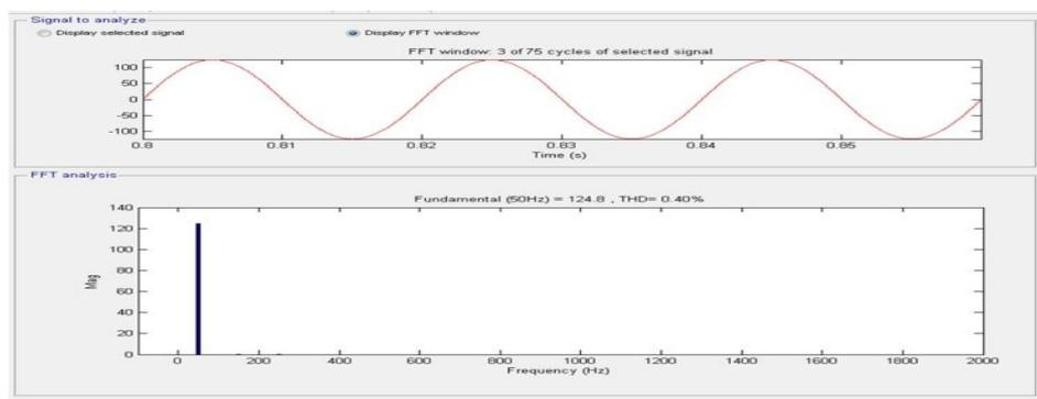
**Fig 5.10:** With STATCOM (a) source current. (b) FFT of source current
