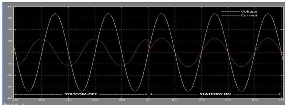
**Fig 5.8:** Supply Voltage and Current at PCC
