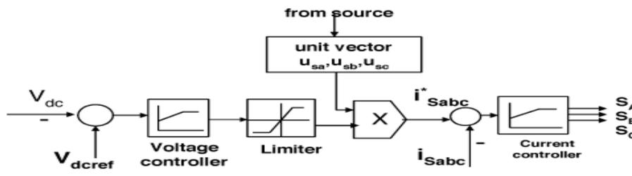
Fig 4.3: Schematic of Bang-Bang Controller
