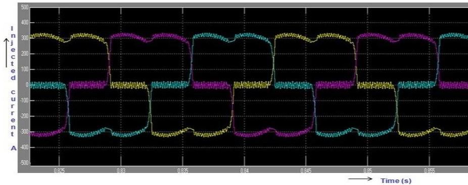
**Fig 5.4:** Three Phase Injected Inverter Current
