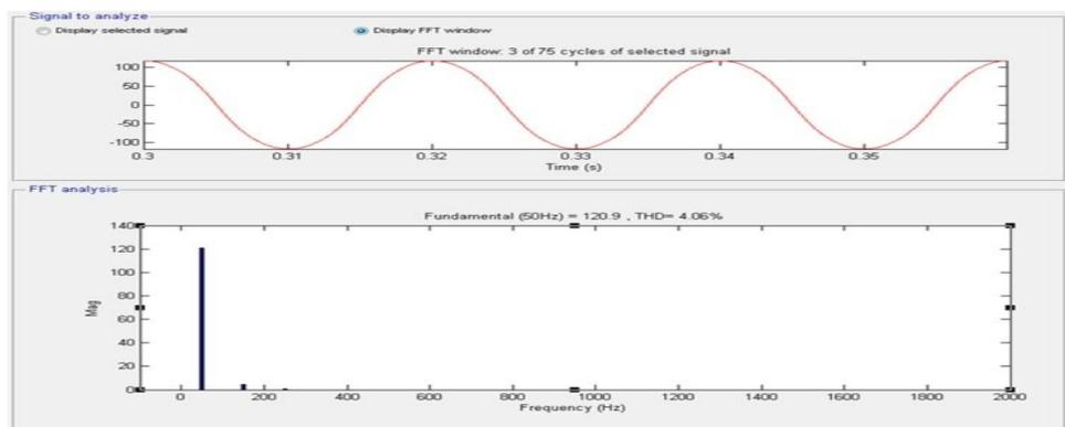
**Fig 5.9:** With out STATCOM (a) source current. (b) FFT of source current
