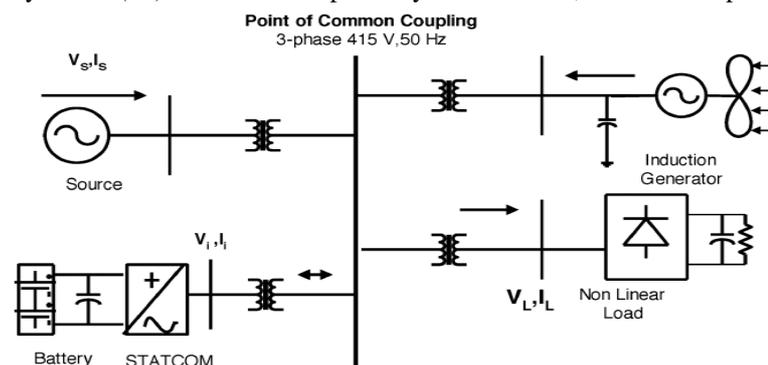
**Fig 4.1:** Grid connected system for power quality improvement
