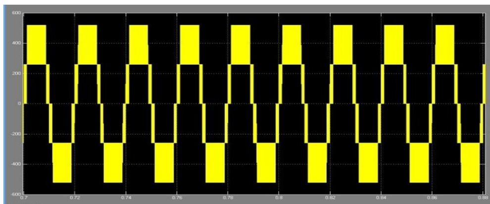
**Fig 5.7:** STATCOM Output Voltage
