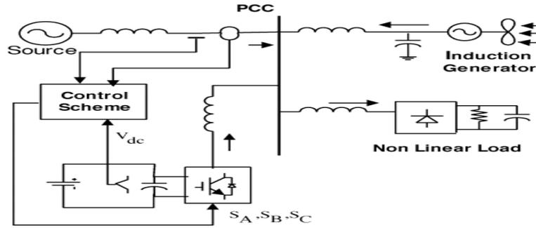
Fig 4.2: System operational scheme in grid system.
